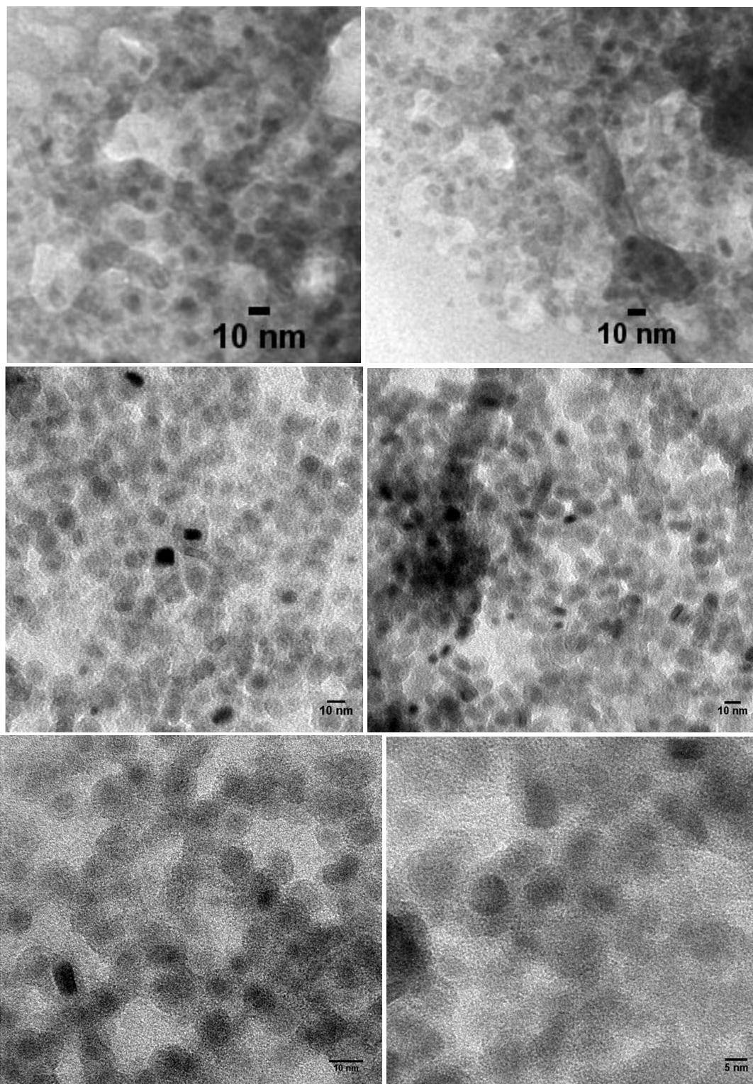
**Figure S1.** Low-resolution TEM images of citrate-capped LaF<sub>3</sub>:Eu(5%) nanocrystals.
