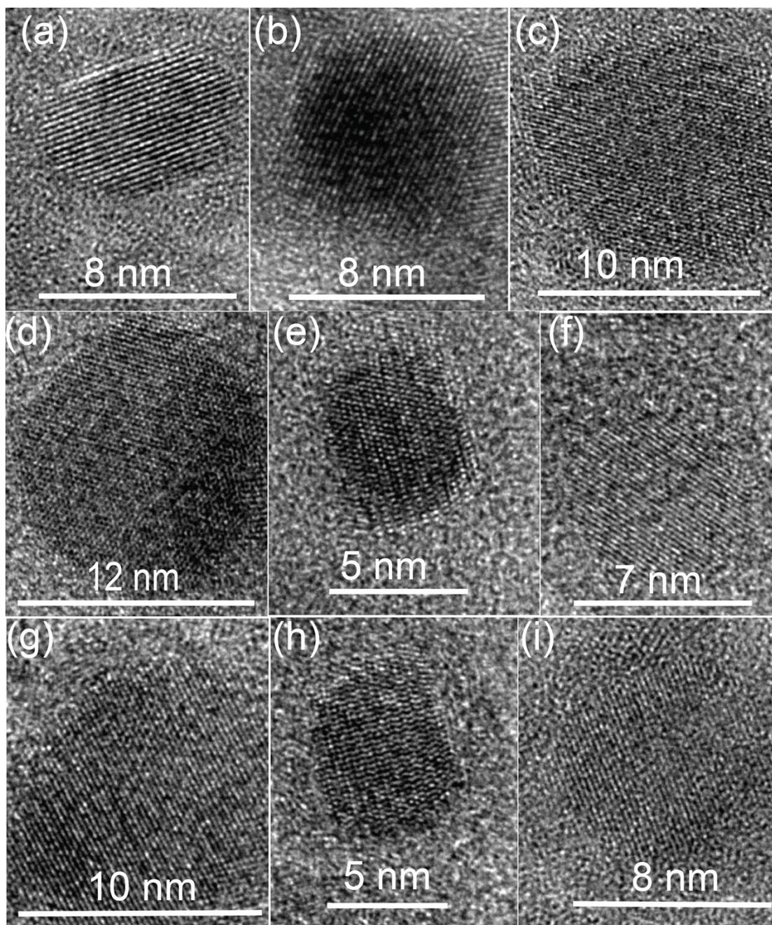
**Figure S2.** Representative high-resolution TEM images of individual citrate-capped  $\text{LaF}_3:\text{Eu}(5\%)$  nanocrystals.
