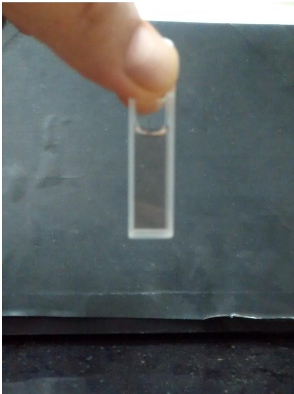
Figure S5. Picture of the colloidal solution of citrate/phen-capped LaF<sub>3</sub>:Eu(5%) NCs in water. The concentration of the colloidal solution is ~50 mg/mL.
