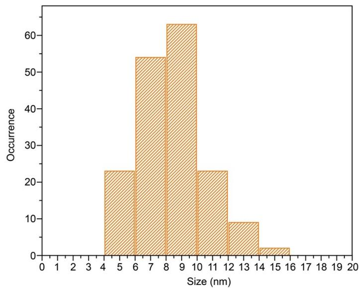
**Figure S3.** TEM size distribution of citrate-capped LaF<sub>3</sub>:Eu(5%) nanocrystals obtained from images of 174 discernible particles.
