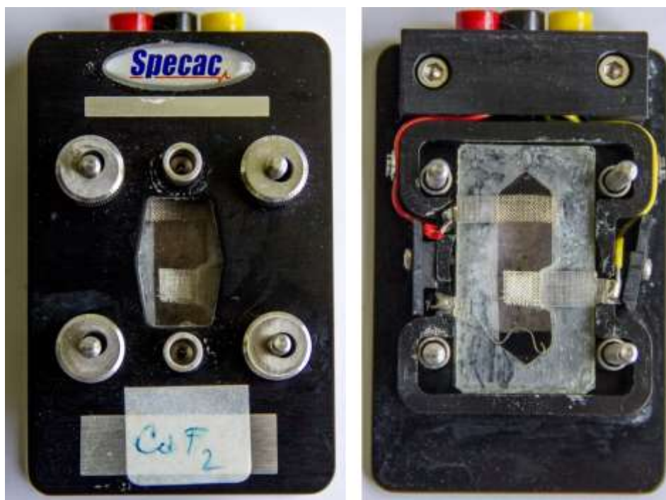
Figure S5. Modified Specac Omni-Cell™ with Platinum net electrode in optical window ( \text{CaF}_2 ), a platinum net as counter electrode and a platinum wire as quasi reference electrode.
