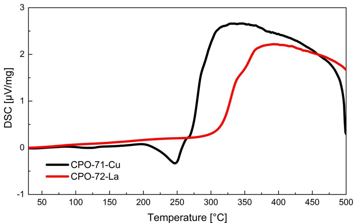
**Figure S 3.** Differential scanning calorimetric analysis of CPO-71-Cu and CPO-72-La. The samples were heated in platinum crucibles at 5K/min in  $\text{N}_2$ .
