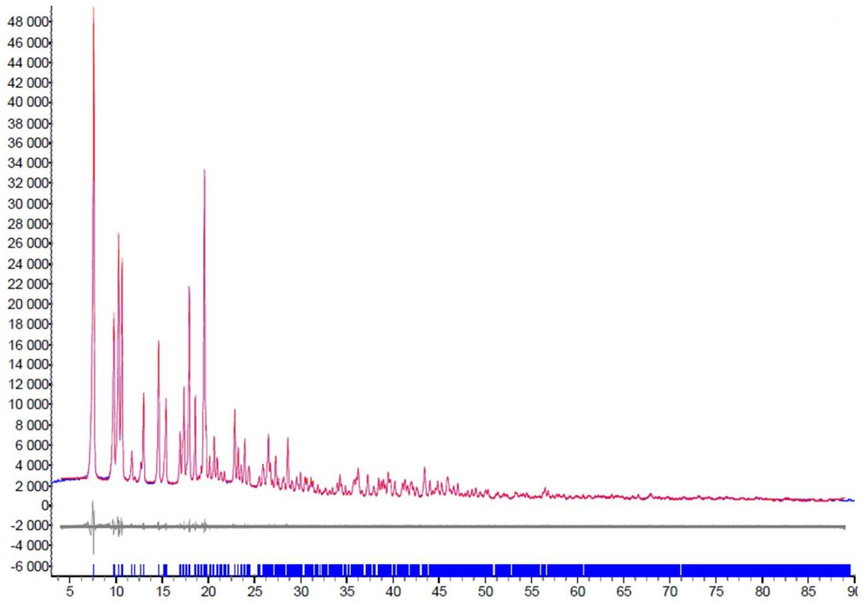
**Figure S 6.** P-XRD and Pawley fit for CPO-71-Cu. P-XRD in blue, simulated pattern in red and difference in grey.  $\lambda = 1.5406 \text{ \AA}$
