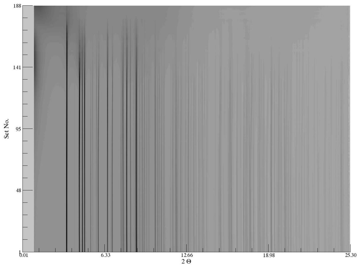
**Figure S 1.** The VT measurement of CPO-71-Cu, y-axis = scan number (increasing temperature), x-axis = reflection angle in degrees  $2\Theta$  ( $\lambda = 0.69396 \text{ \AA}$ ).
