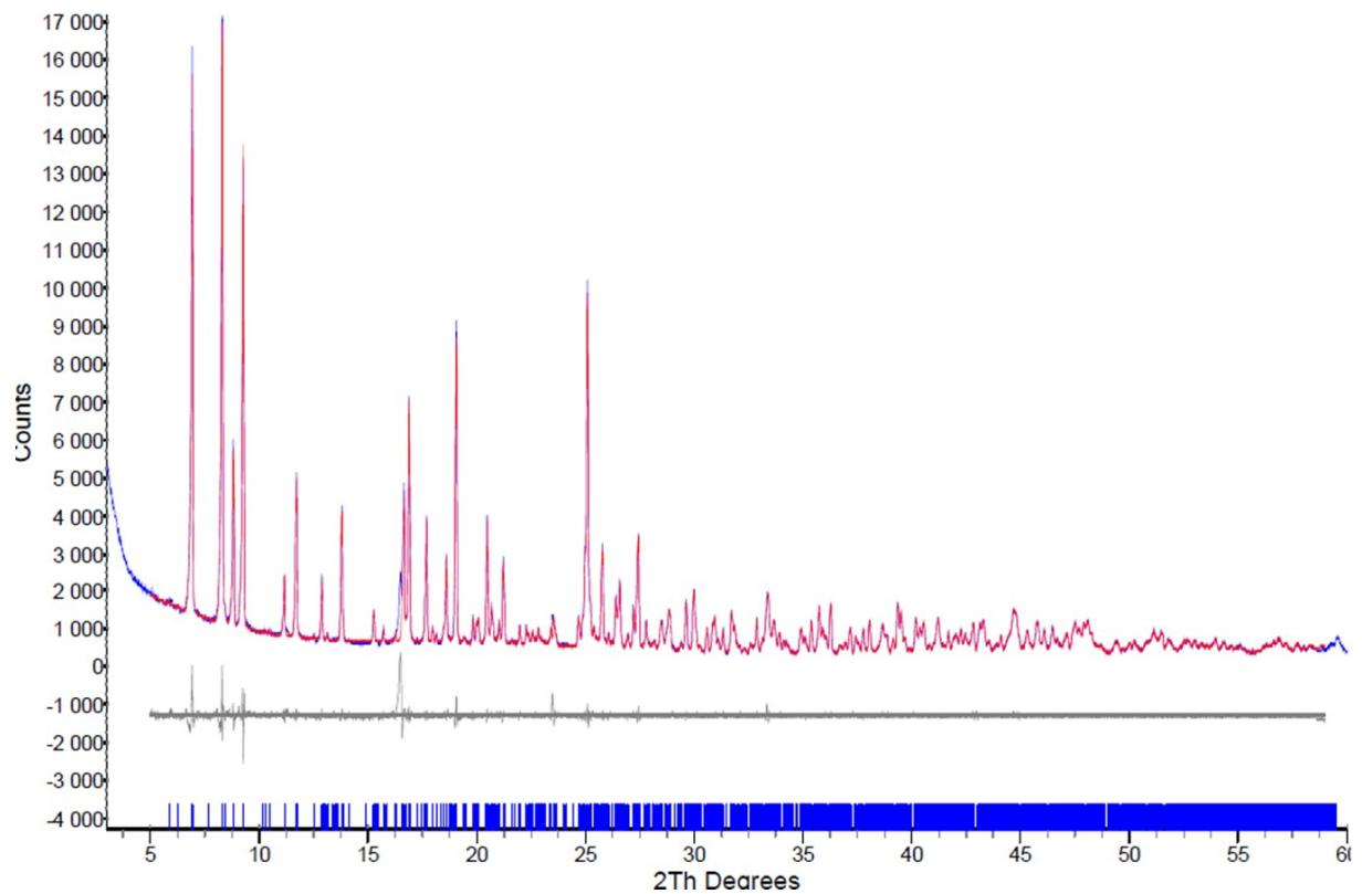
**Figure S 7.** P-XRD and Pawley fit for CPO-72-La. P-XRD in blue, simulated pattern in red and difference in grey.  $\lambda = 1.5406 \text{ \AA}$
