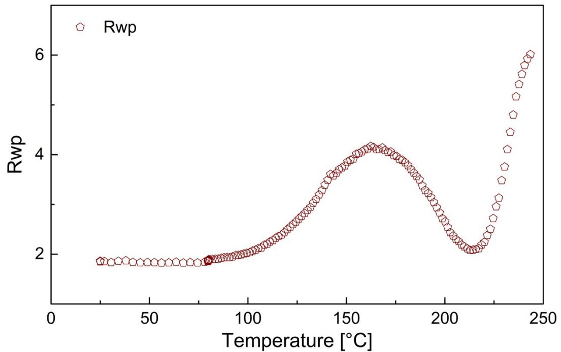
**Figure S 4.** Rwp from the parametric refinement of CPO-71-Cu plotted against temperature.
