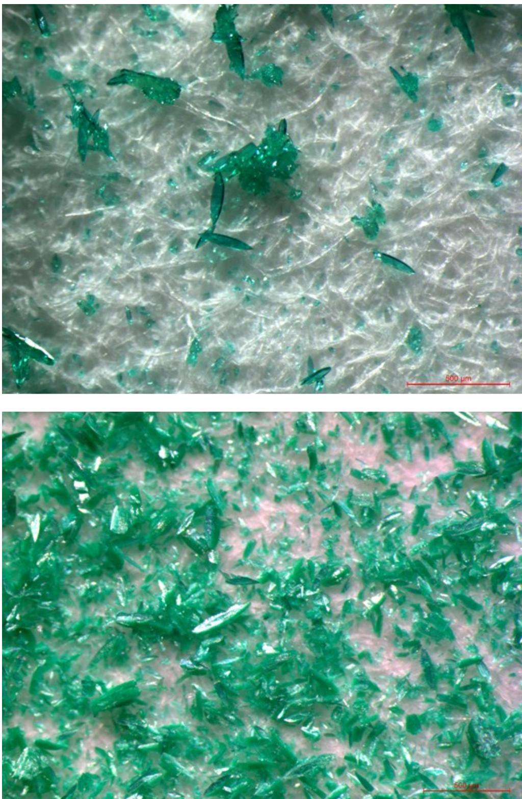
**Figure S 8.** Microscope images of CPO-71-Cu before (top) and after (bottom) solvent exchange with methanol for 48 hours. The red scale bar is set to 500  $\mu\text{m}$  in both images.
