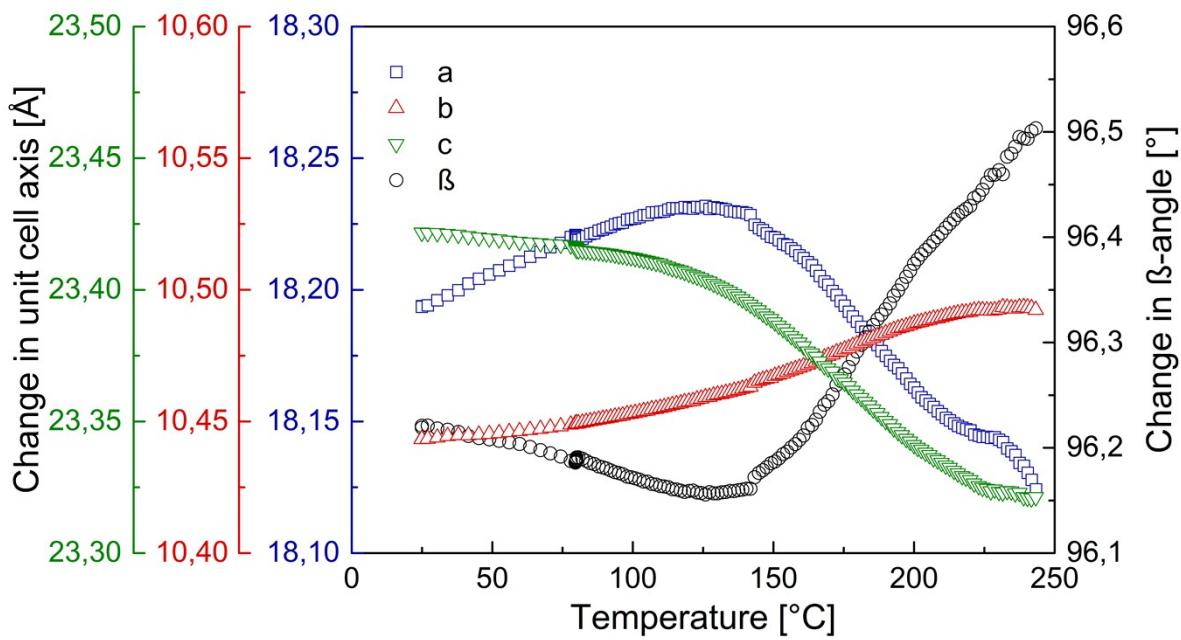
**Figure S 5.** Unit cell parameters of CPO-71-Cu extracted from the parametric refinement of the variable temperature P-XRD experiment.
