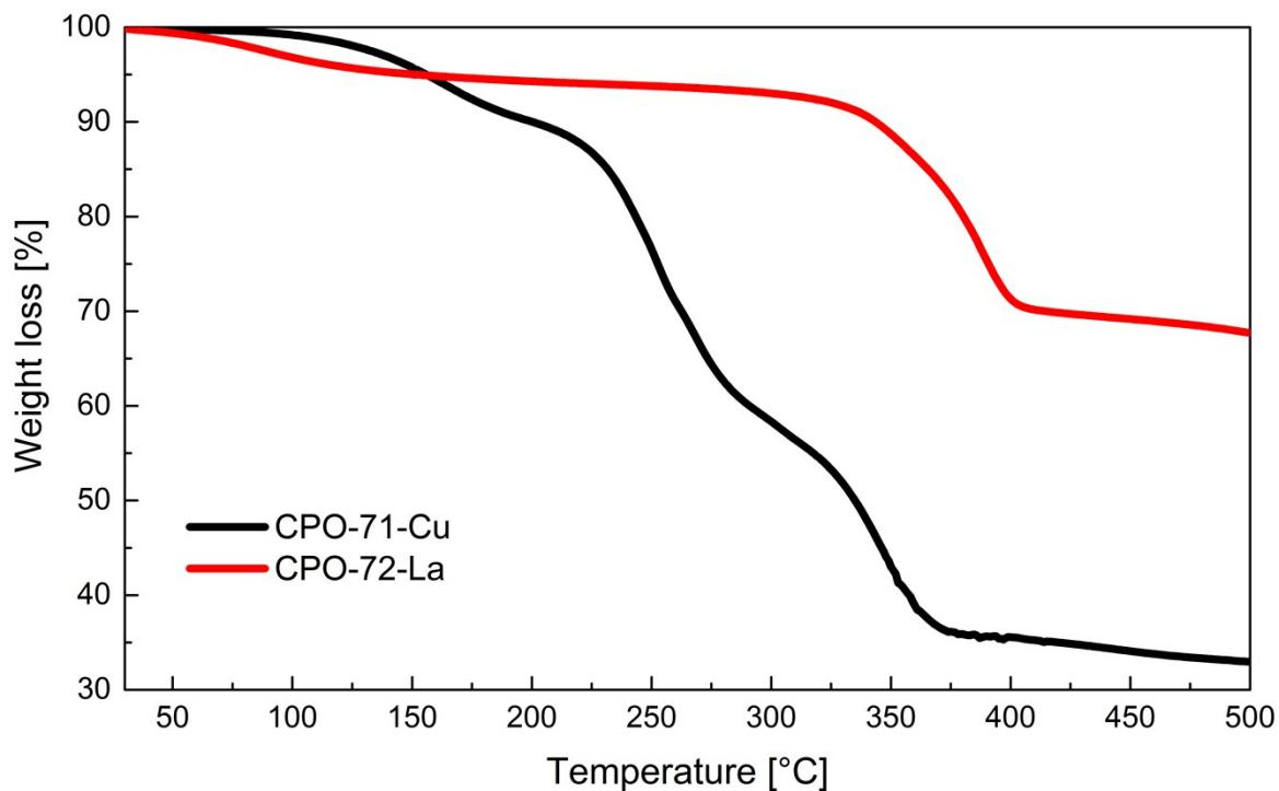
**Figure S 2.** Thermogravimetric analysis of CPO-71-Cu and CPO-72-La. The samples were heated in alumina crucibles at 2K/min in N<sub>2</sub>.
