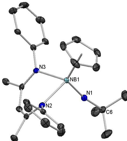
**Figure S12:** Molecular structure of **5** as determined by X-ray diffraction. Hydrogen atoms, a second equivalent molecule of **5**, and aryl isopropyl groups have been omitted for clarity; thermal ellipsoids are set at the 50% probability level. Selected bond lengths (Å): Nb(1)-N(1) 1.794(2), Nb(1)-N(2) 2.210(2), Nb(1)-N(3) 2.207(2). Selected bond angles (°): C(6)-N(1)-Nb(1) 168.07(2), N(2)-Nb(1)-N(3) 83.68(8).
