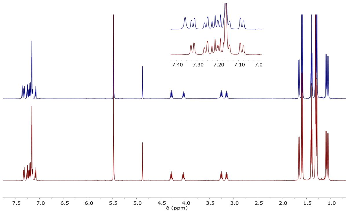
**Figure S9:** Stacked spectra of **6** (blue, top) and **6-D** (red, bottom) with the aromatic region enlarged, showing the chemical shift for the Nb-*H* that appears at 7.36 ppm for **6** and is absent in the spectrum of **6-D**.
