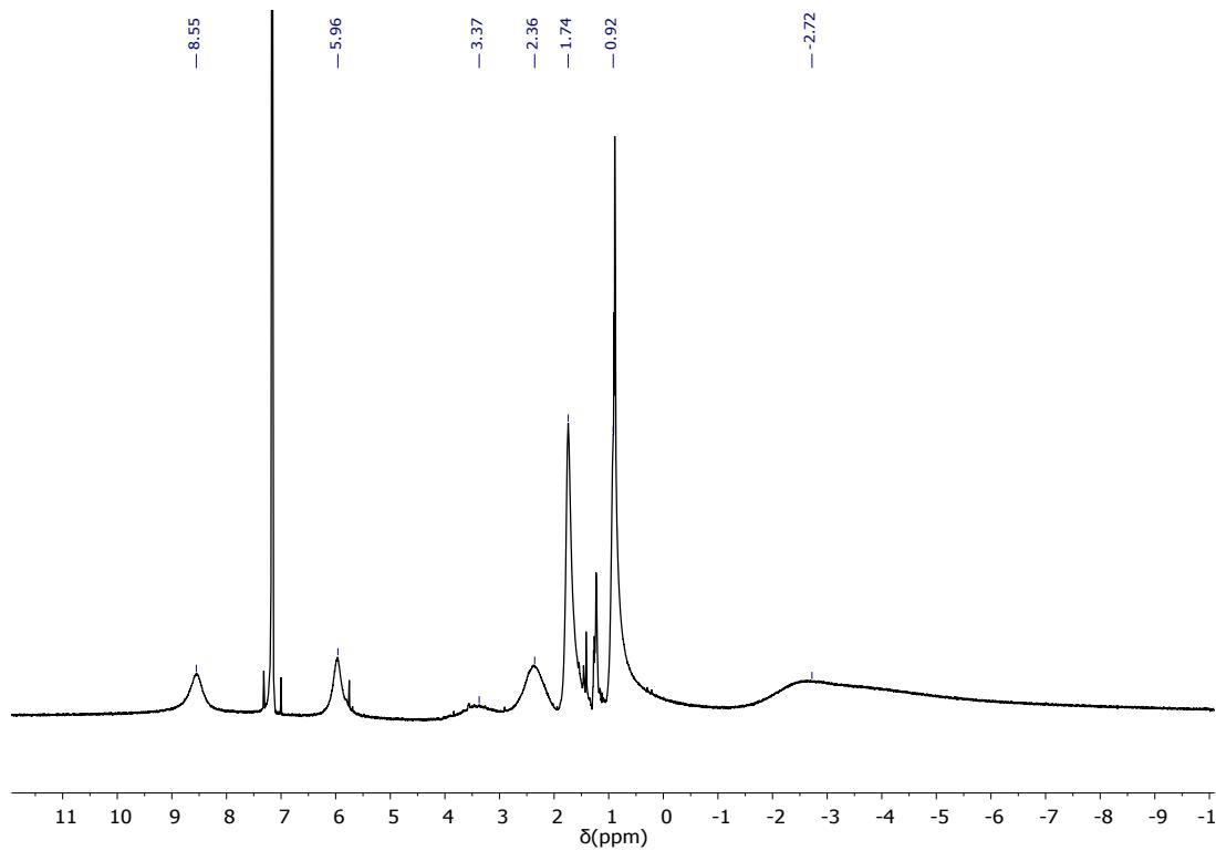
**Figure S7:**  $^1\text{H}$  NMR spectrum of paramagnetic complex **5** in  $\text{C}_6\text{D}_6$  at room temperature.
