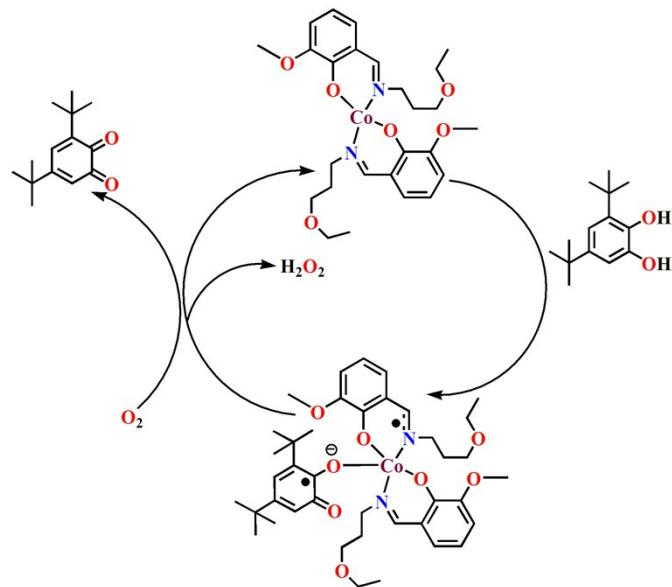
**Scheme S2.** Proposed mechanism for the catalytic cycle of 3,5-DTBCH<sub>2</sub> oxidation by Co(II) complexes.
