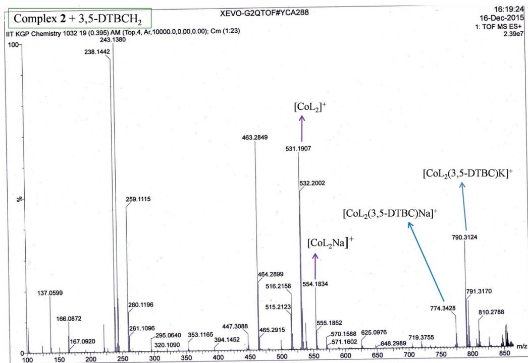
**Fig. S13.** Electrospray mass spectrum (ESI-MS positive) of **2** and 3,5-DTBCH<sub>2</sub> (1:100) in MeCN after 20 min of mixing
