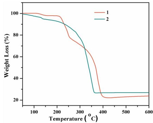
**Fig. S6.** Thermograms for **1–2** in air up to 600 °C
