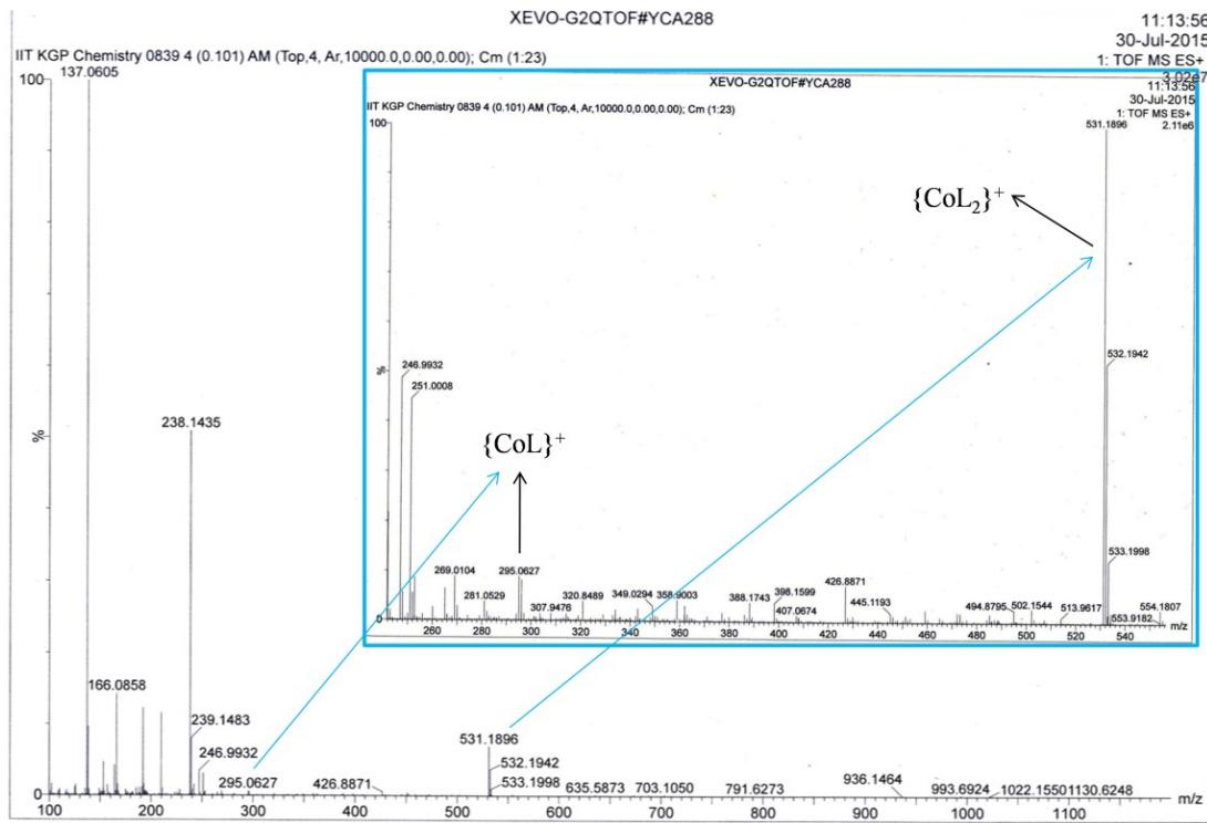
**Fig. S1.** Electrospray mass spectrum (ESI-MS positive) of **1** in MeOH solution
