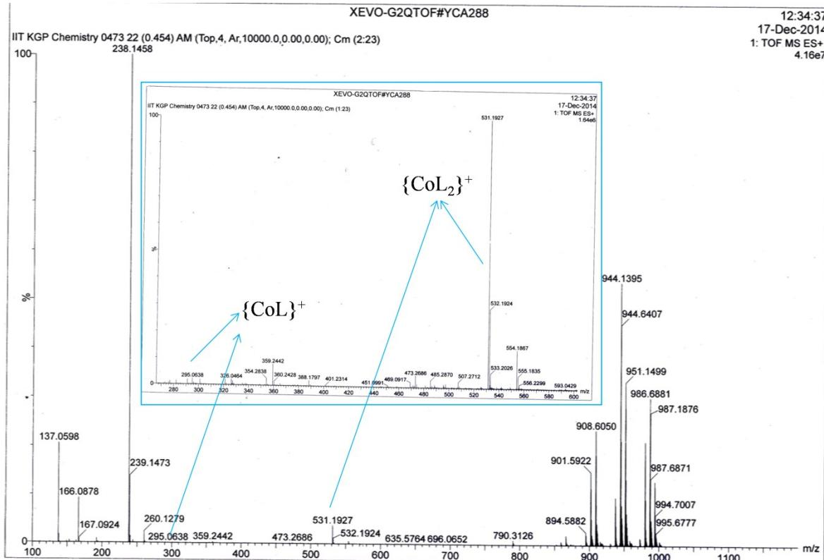
**Fig. S2.** Electrospray mass spectrum (ESI-MS positive) of **2** in MeOH solution
