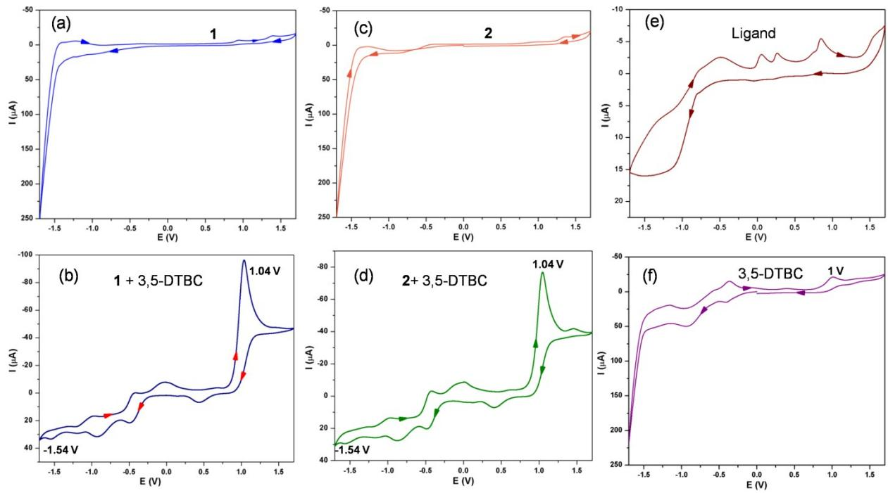
**Fig. S14.** Cyclic voltammogram of (a) **1** ( $10^{-4}$  M), (b) **1+3,5 DTBCH<sub>2</sub>** ( $10^{-2}$  M) (c) **2** ( $10^{-4}$  M), (d) **2+3,5 DTBCH<sub>2</sub>** ( $10^{-2}$  M), (e) ligand ( $10^{-3}$  M) and (f) **3,5 DTBCH<sub>2</sub>** ( $10^{-3}$  M) in MeCN using 0.1 M [<sup>n</sup>Bu<sub>4</sub>][ClO<sub>4</sub>] as the supporting electrolyte, a Pt disc working electrode and a Ag/AgCl reference electrode with scan rate at of 50 mV s<sup>-1</sup>
