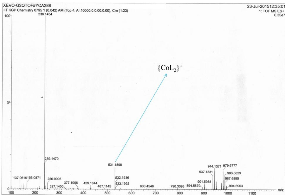
**Fig. S11.** Electrospray mass spectrum (ESI-MS positive) of **2** in MeCN solution
