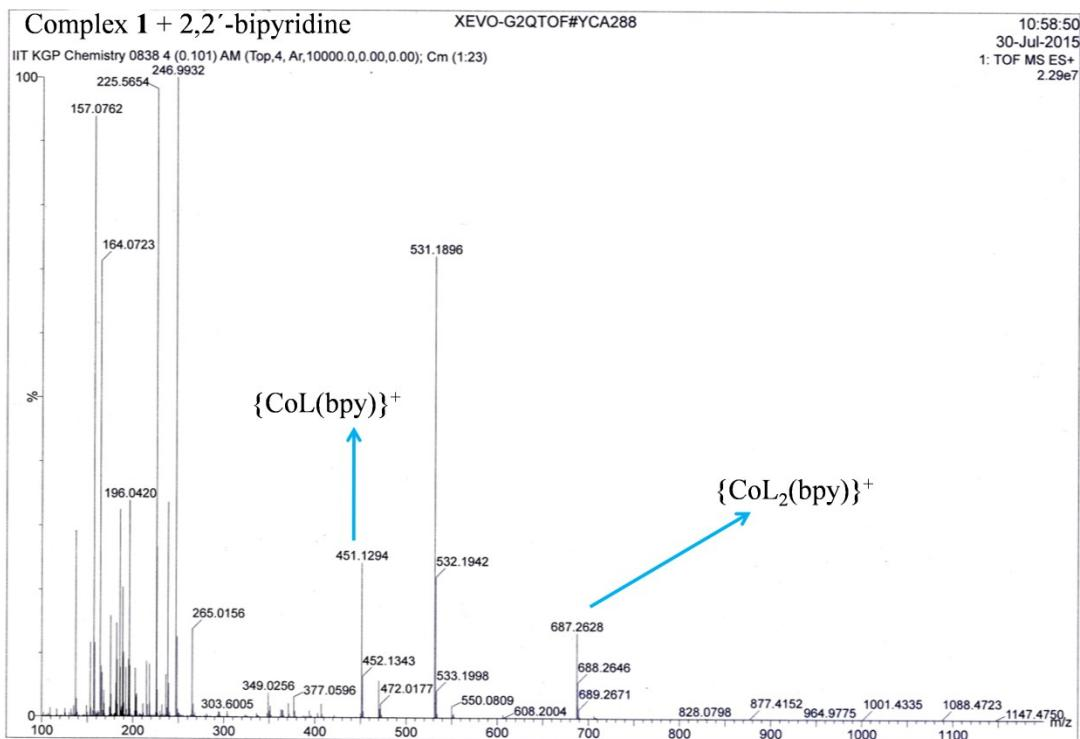
**Fig. S3.** Electrospray mass spectrum (ESI-MS positive) of **1** with 2,2'-bipyridine in 1:1 mole ratio in MeOH solution
