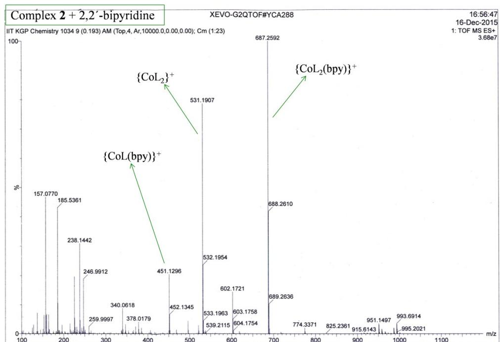
**Fig. S4.** Electrospray mass spectrum (ESI-MS positive) of **2** with 2,2'-bipyridine in 1:1 mole ratio in MeOH solution
