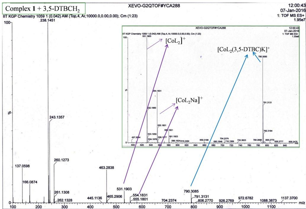
**Fig. S12.** Electrospray mass spectrum (ESI-MS positive) of **1** and 3,5-DTBCH<sub>2</sub> (1:100) in MeCN after 20 min of mixing
