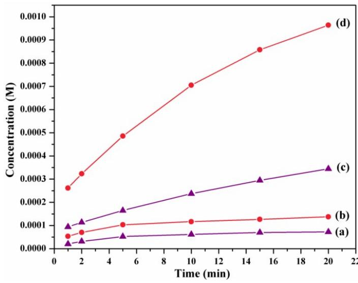
**Fig. S9.** Change in concentrations of H<sub>2</sub>O<sub>2</sub> (a and b) and 3,5-DTBQ (c and d) during the catalytic reaction of 3,5-DTBCH<sub>2</sub> with **1** and **2**, respectively
