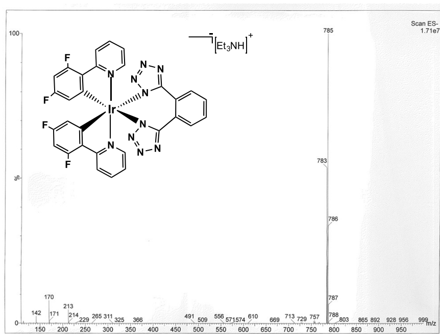
Figure S2: ESI-MS spectrum of [\text{Ir}(\text{F}_2\text{ppy})_2(1,2\text{ BTB})]^- (negative ions region) [\text{M}]^- = 785\text{ m/z} , \text{CH}_3\text{CN} .
