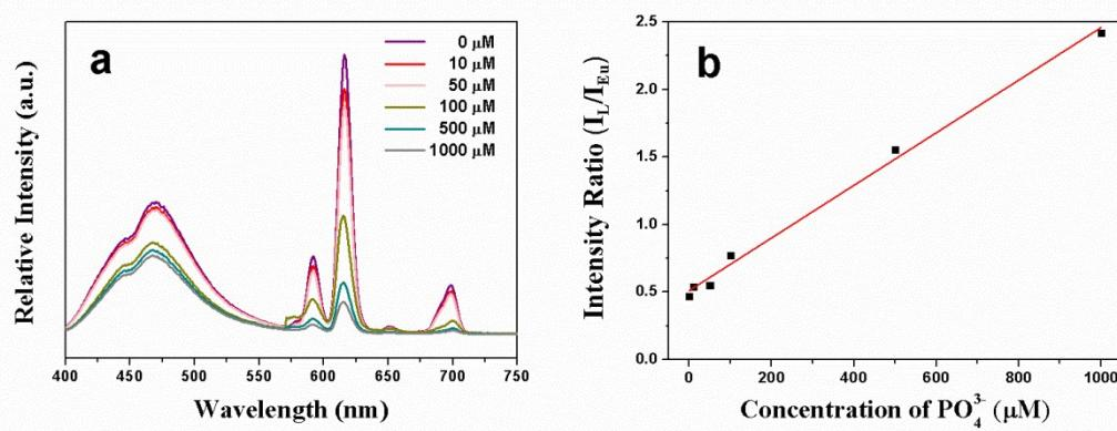
**Fig. S8** (a) The emission spectra of MIL-125(Ti)-AM-Eu immersed in PO<sub>4</sub><sup>3-</sup> solvents with different concentrations from 0 μM to 1000 μM; (b) the plot of the intensity ratio of <sup>5</sup>D<sub>0</sub> → <sup>7</sup>F<sub>2</sub> transition of Eu<sup>3+</sup> and the ligand emission ( $I_L/I_{Eu}$ ) as a function of concentration (μM) of PO<sub>4</sub><sup>3-</sup>.
