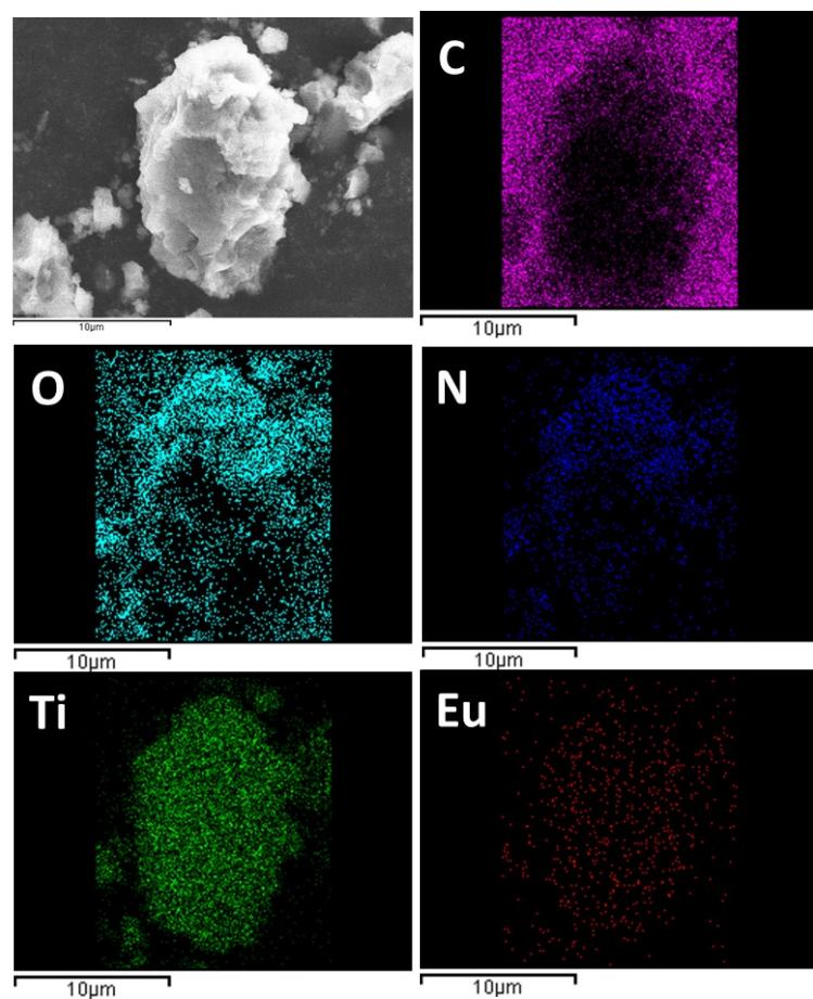
**Fig. S6** The EDX-Mapping images of MIL-125(Ti)-AM-Eu for different elements (C, O, N, Ti, Eu).
