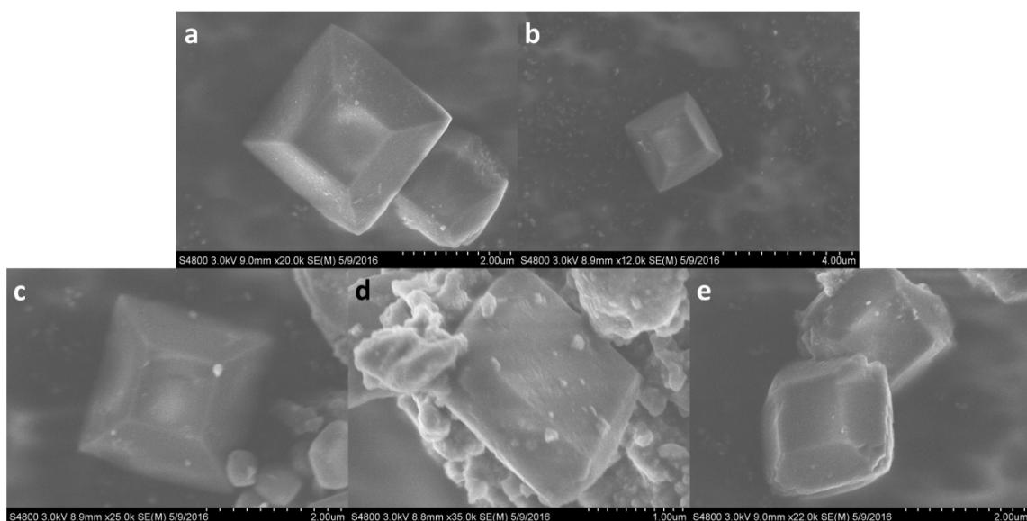
**Fig. S2** Selected SEM images of as-prepared MIL-125(Ti)-NH<sub>2</sub> (a-b), MIL-125(Ti)-AM (c-d) and MIL-125(Ti)-AM-Eu (e).
