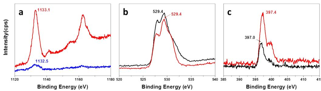
**Fig. S7** (a) XPS spectra of MIL-125(Ti)-AM-Eu (blue) and Eu(No<sub>3</sub>)<sub>3</sub>·6H<sub>2</sub>O (red) for Eu 3d and Eu 4d; XPS spectra of MIL-125(Ti)-AM (black) and MIL-125(Ti)-AM-Eu (red): (b) O 1s and (c) N 1s.
