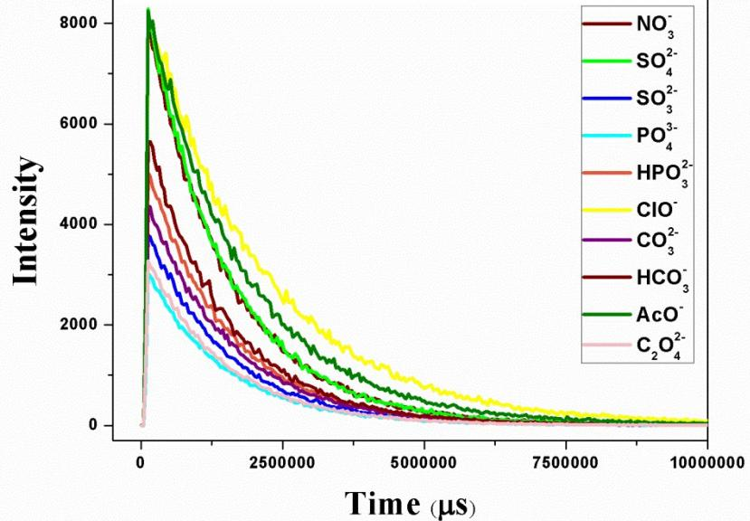
**Fig. S10** The luminescence decay times ( ${}^5\text{D}_0 \rightarrow {}^7\text{F}_2$ ) of MIL-125(Ti)-AM-Eu after the adsorption of different anions. The excitation wavelength is 255 nm.
