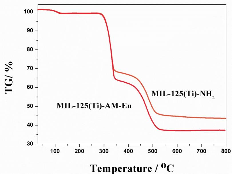
**Fig. S5** Thermal gravimetric analysis (TGA) curves of MIL-125(Ti)-NH<sub>2</sub> and MIL-125(Ti)-AM-Eu.
