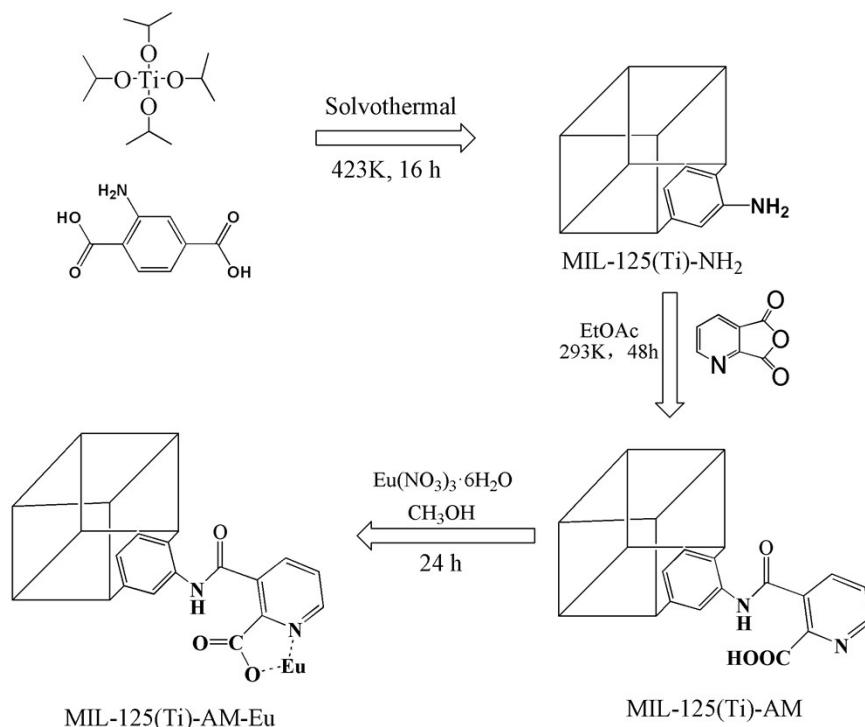
**Fig. S1** Schematic of synthesis of MIL-125(Ti)-AM-Eu. The solvent molecules (include DMF and H<sub>2</sub>O) and three nitrates for balance charge which could coordinate with Eu(III) were omitted for simplicity.
