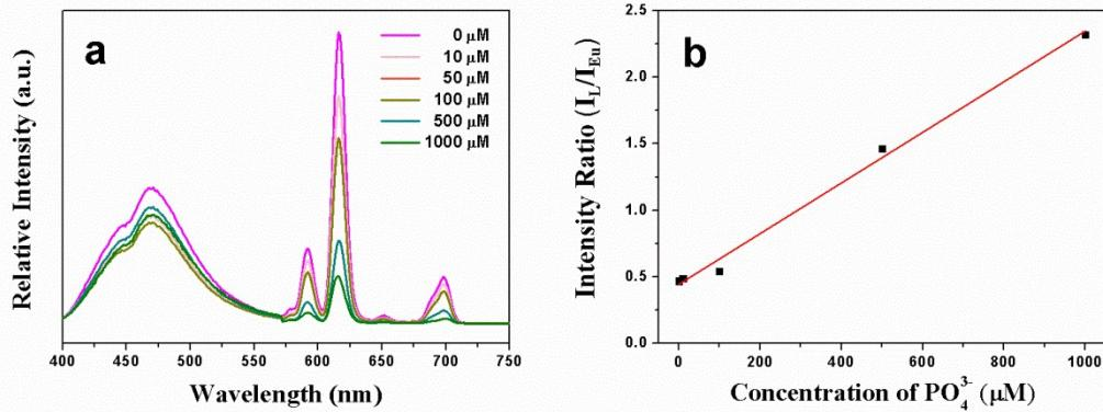
**Fig. S9** (a) The emission spectra of MIL-125(Ti)-AM-Eu immersed in  $\text{C}_2\text{O}_4^{2-}$  solvents with different concentrations from 0  $\mu\text{M}$  to 1000  $\mu\text{M}$ ; (b) the plot of the intensity ratio of  ${}^5\text{D}_0 \rightarrow {}^7\text{F}_2$  transition of  $\text{Eu}^{3+}$  and the ligand emission ( $I_L/I_{\text{Eu}}$ ) as a function of concentration ( $\mu\text{M}$ ) of  $\text{C}_2\text{O}_4^{2-}$ .
