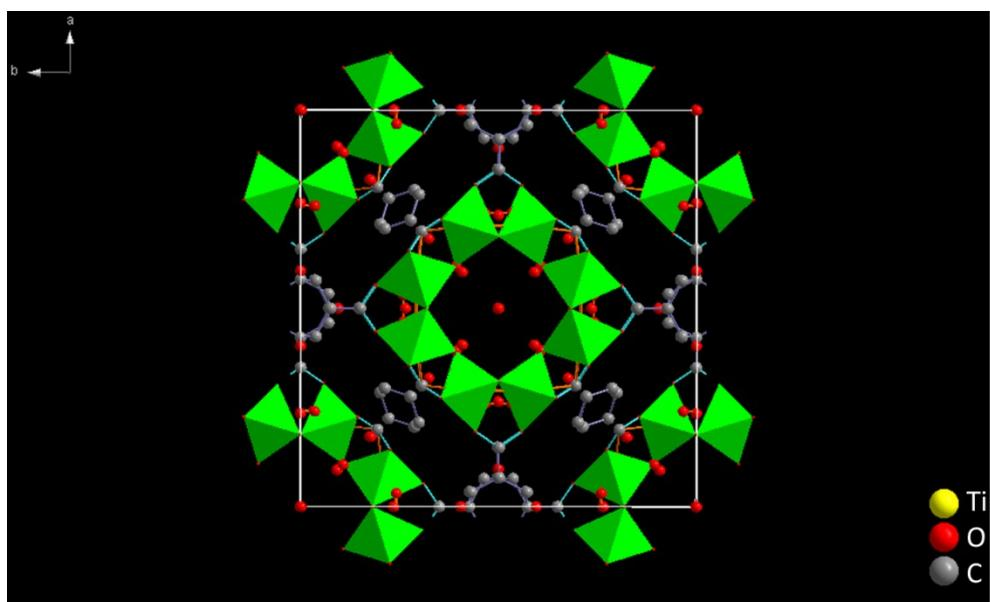
**Scheme S1** The structure and typical coordination environment of MIL-125(Ti)-NH<sub>2</sub>.
