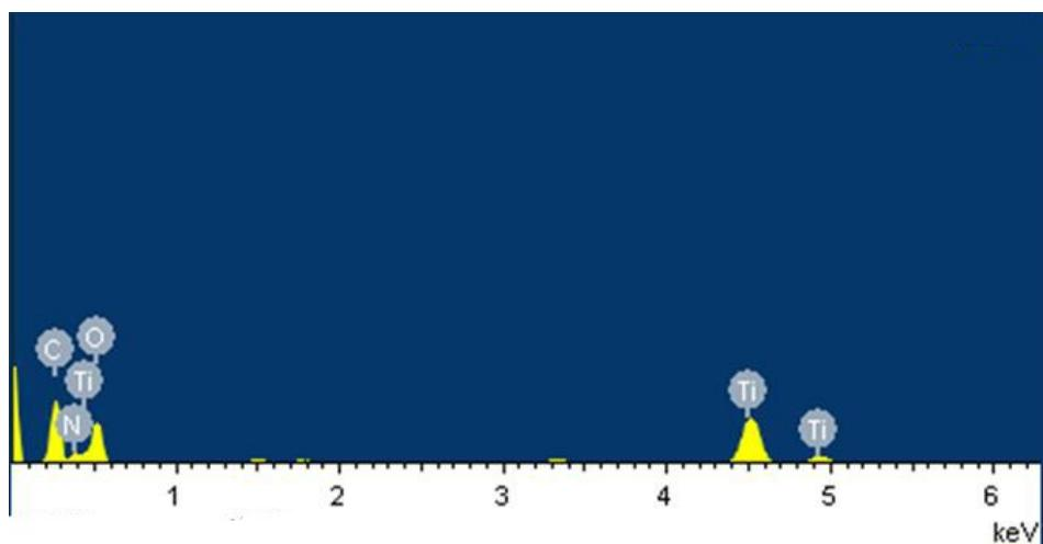
**Fig. S3** Energy dispersive analysis by X-rays (EDX) spectroscopy of MIL-125(Ti)-NH<sub>2</sub>.
