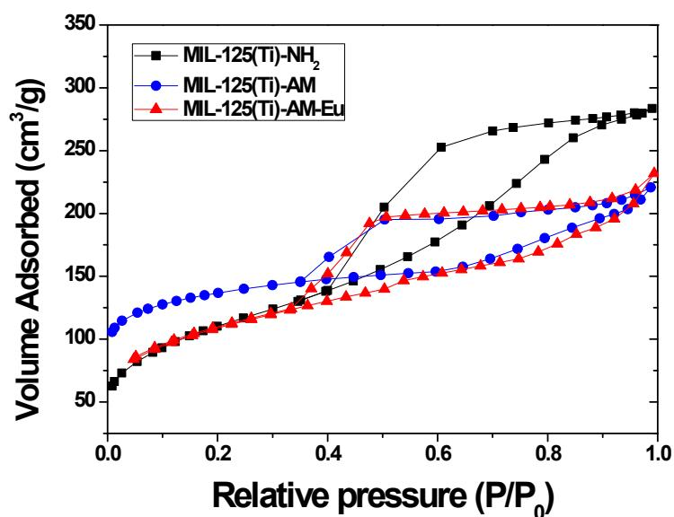
**Fig. S4** The N<sub>2</sub> adsorption–desorption isotherms of MIL-125(Ti)-NH<sub>2</sub>, MIL-125(Ti)-AM and MIL- 125(Ti)-AM-Eu.
