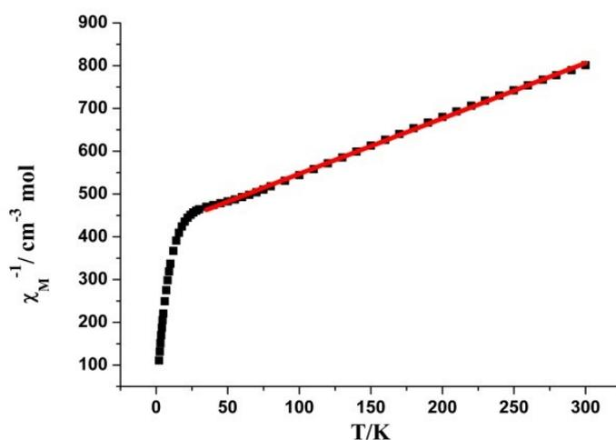
**Figure S10.** The temperature dependence of the inverse magnetic susceptibility  $\chi_M^{-1}$  for **VMOP-17** between 2 and 300 K. The solid red line was generated from the best fit by the Curie-Weiss expression in the range of 35–300 K.
