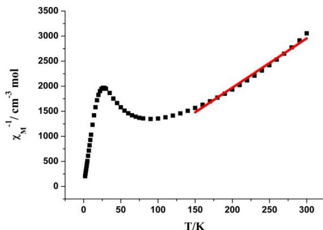
**Figure S9.** The temperature dependence of the inverse magnetic susceptibility  $\chi_M^{-1}$  for **VMOP-16** between 2 and 300 K. The solid red line was generated from the best fit by the Curie-Weiss expression in the range of 150–300 K.
