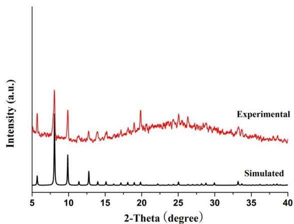
**Figure S2.** Experimental and simulated powder X-Ray diffraction patterns for VMOP-16.
