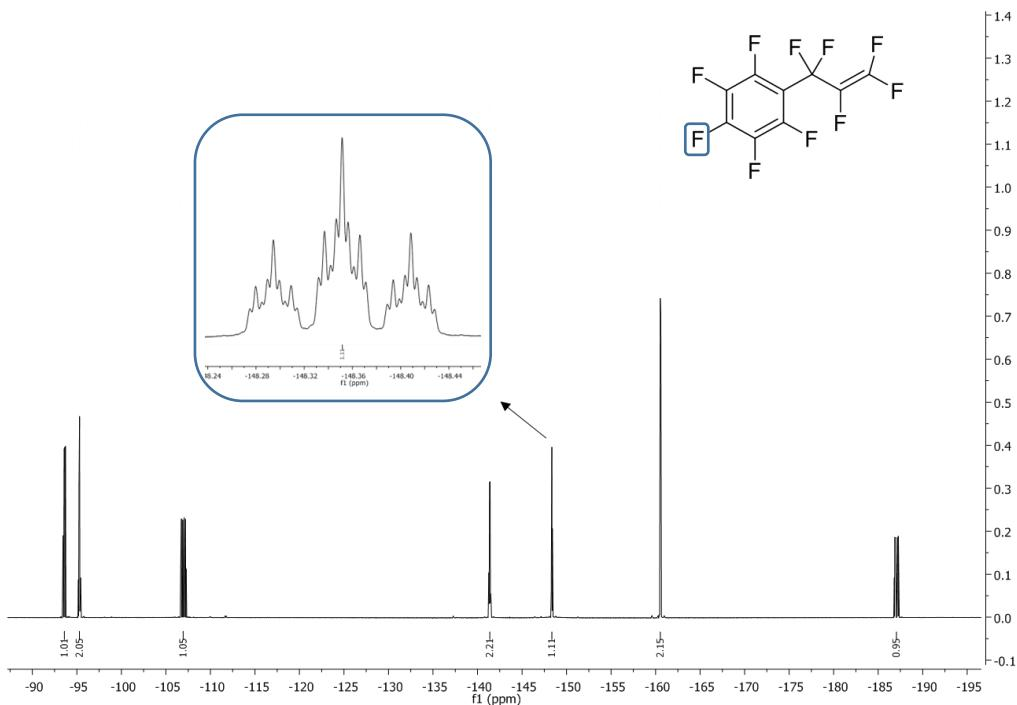
**Figure S1:** <sup>19</sup>F NMR of perfluorallylbenzene, resonance of the *para*-fluorine nuclei expanded.
