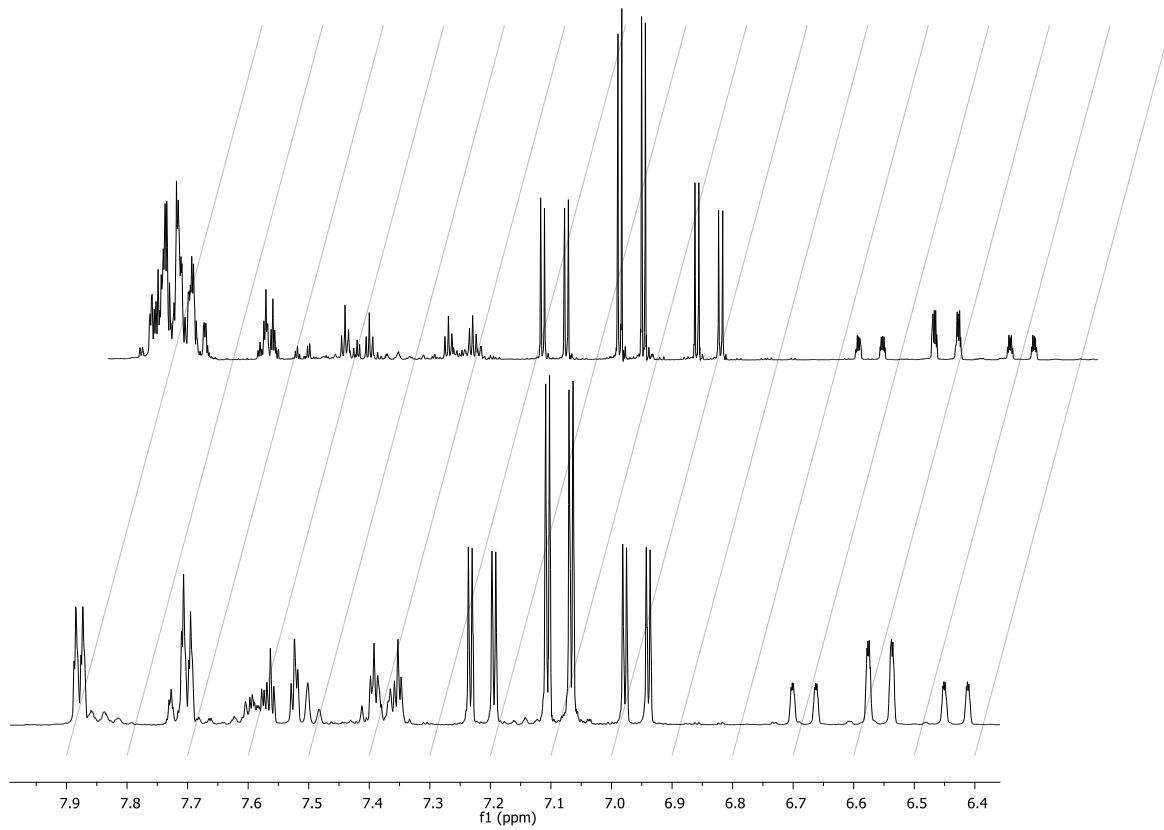
**Figure S4.** <sup>1</sup>H NMR spectra of a reaction mixture containing mainly *top*: 1<sup>st</sup> generation HDF products (**4a, b, c, d**) and *bottom*: 2<sup>nd</sup> generation products (**4a', b', c', d'**), additional resonances of the aromatic protons are observed at low field.
