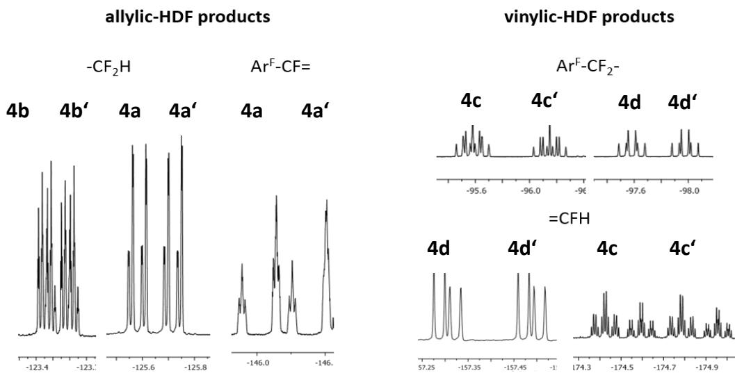
**Figure S3.** Selection of the doubled characteristically signals for **4a, a', b, b', c, c', d, d'**.
