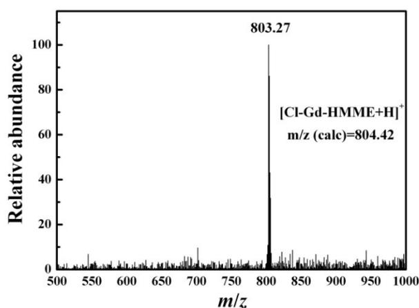
Figure S1. Basic characterization for Gd-HMME by mass spectroscopy.
