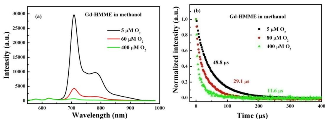
Figure S4. Luminescence spectra and phosphorescence decay profiles for Gd-HMME in the presence of various concentrations of oxygen.
