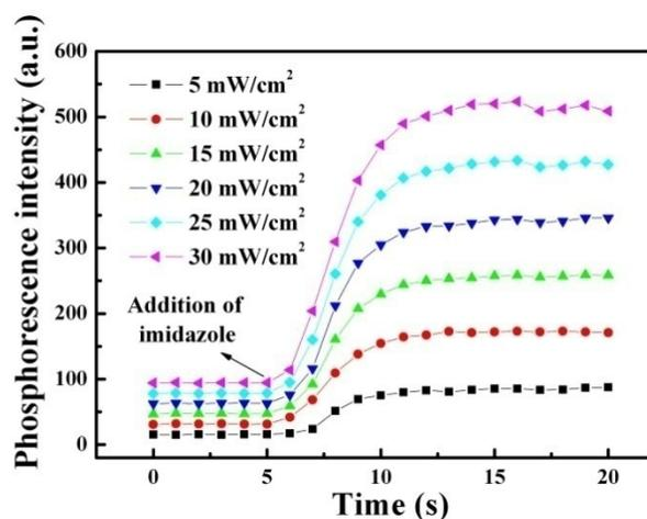
Figure S5. The time dependences of the phosphorescence intensity of Gd-HMME upon addition of imidazole under various excitation power density from 5 to 30 mW/cm<sup>2</sup>.
