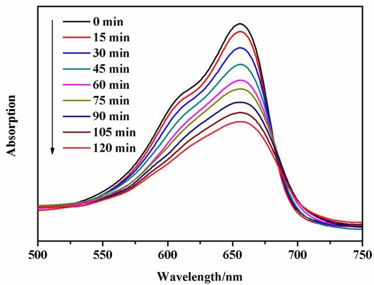
**Fig. S9** Absorption spectra of the MB solution during the photodegradation reaction under UV irradiation in the presence of CP 1 and TBA.
