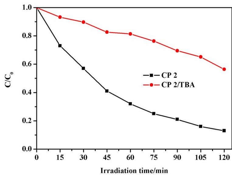
**Fig. S12** Photocatalytic degradation of the MB solution under UV irradiation with the use of CP 2 and CP 2 in the presence of TBA.
