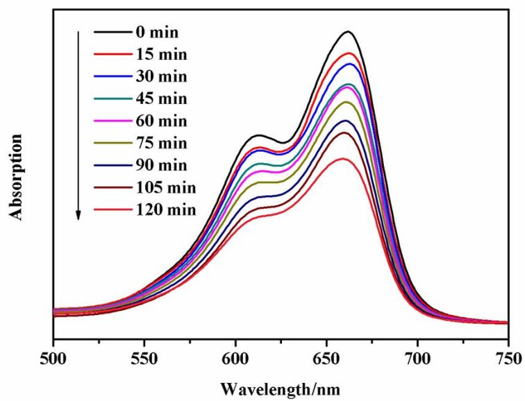
**Fig. S11** Absorption spectra of the MB solution during the photodegradation reaction under UV irradiation in the presence of CP 2 and TBA.
