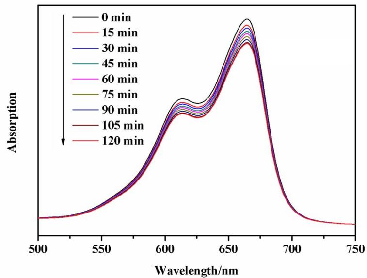
**Fig. S8** Absorption spectra of the MB solution during the photodegradation reaction under UV irradiation without catalyst.
