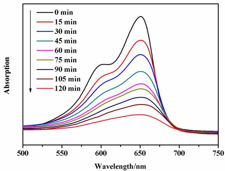
**Fig. S13** Absorption spectra of the Congo red solution during the photodegradation reaction under UV irradiation in the presence of CP 1.
