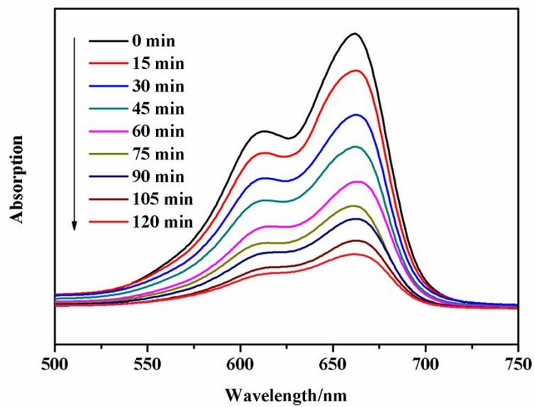
**Fig. S14** Absorption spectra of the Congo red solution during the photodegradation reaction under UV irradiation in the presence of CP 2.
