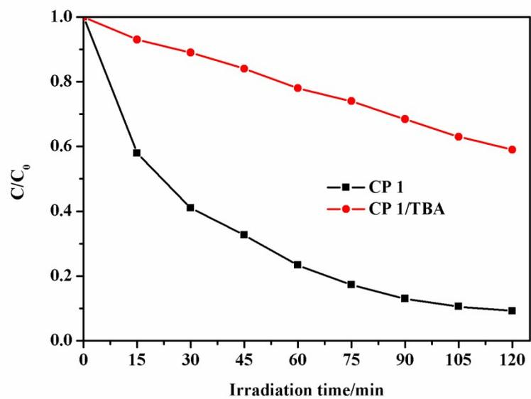
**Fig. S10** Photocatalytic degradation of the MB solution under UV irradiation with the use of CP 1 and CP 1 in the presence of TBA.
