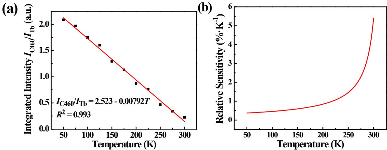
Fig. S11 (a) Temperature-dependent integrated intensity ratio of C460 (385-480 nm) to Tb<sup>3+</sup> (535-560 nm) and the fitted curve for TbTATAB=C460. (b) Temperature-dependent relative sensitivity ( $S_r$ ) of TbTATAB=C460.
