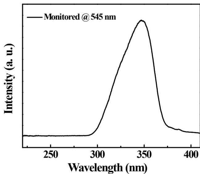
Fig. S4 Excitation spectra of TbTATAB monitored at 545 nm.
