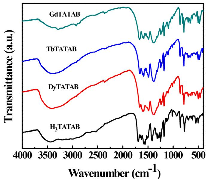
Fig. S3 FT-IR spectra of H<sub>3</sub>TATAB and LnTATAB (Ln = Dy, Tb, and Gd).
