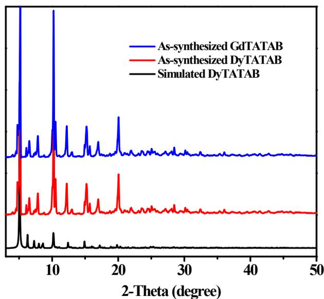
**Fig. S2** PXRD patterns of as-synthesized DyTATAB and GdTATAB.
