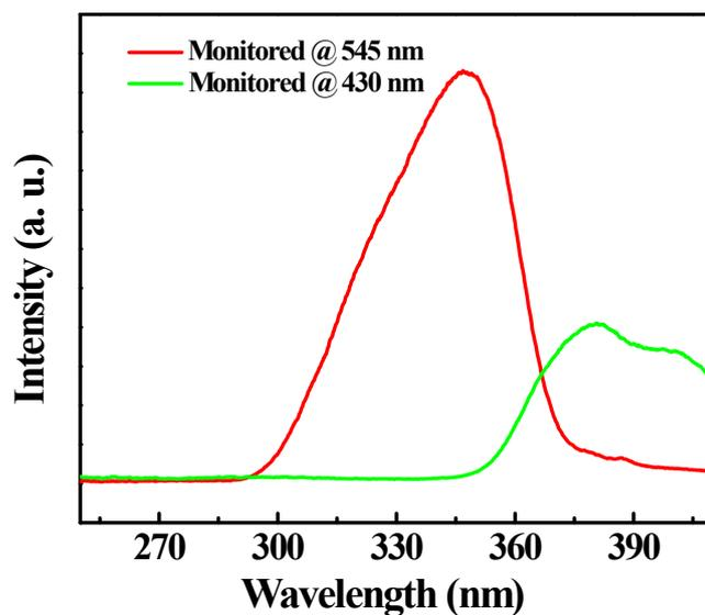
Fig. S6 Excitation spectra of TbTATAB=C460 monitored at 430 nm and 545 nm, respectively.
