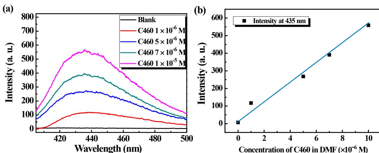
Fig. S12 (a) The intensity of C460 in DMF with different concentrations and (b) the fitted curve between the intensity and the concentration.
