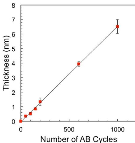
**Figure S9:** Correlation of film thickness vs. number of ALD “A-B” cycles of precursor **3** and O<sub>3</sub> as grown on Si wafers measured ex-situ using spectroscopic ellipsometry. A timing sequence (t<sub>1</sub>–t<sub>2</sub>–t<sub>3</sub>–t<sub>4</sub>) of 2–30–10–45 was used at a reactor temperature of 150 °C.
