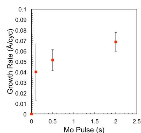
**Figure S8:** Growth rate as a function of the pulse time of precursor **3**. Large fluctuations of measured thicknesses were observed at lower pulse times due to lack of precursor vapor to fully saturate and react with the surface of the silicon wafers.
