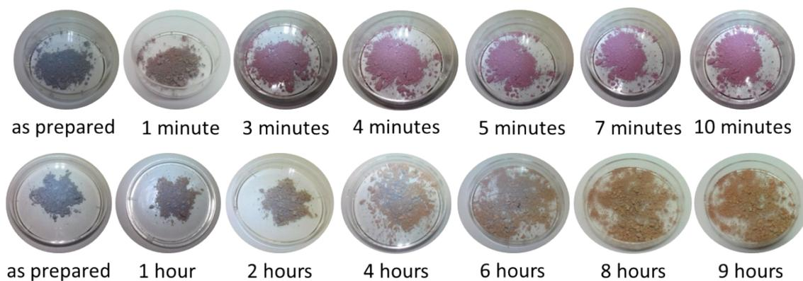
Fig. S11. Photographs of powdered sample of  $\mathbf{1@BaSO_4}$  in vapors of 7M (top) and 2M (bottom) HCl.
