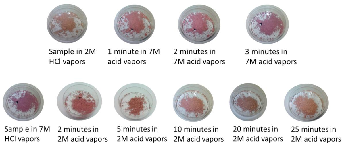
Fig. S14. Gradual changes of color over the time of **1@BASO<sub>4</sub>** sample from 2M HCl to 7M HCl (top) and from 7M HCl to 2M HCl (bottom).
