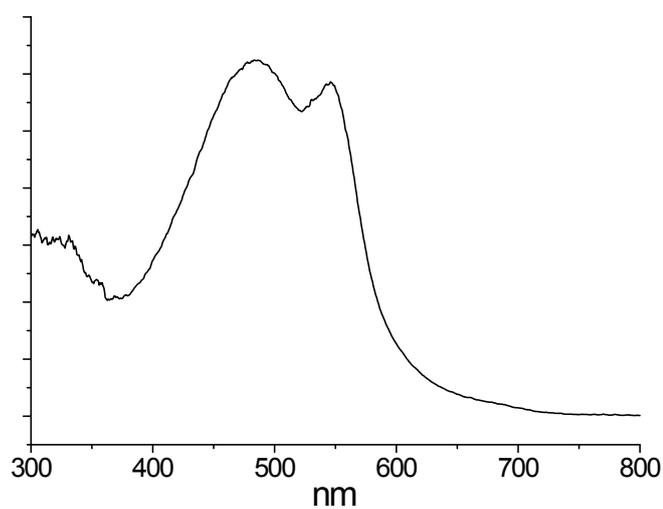
Fig. S12. Diffuse reflectance spectra of  $\mathbf{1@BaSO_4}$  saturated in the vapours of 5M HCl. The spectrum comprises two components at 480 ( $H_3L$  form) and 550 nm ( $H_4L^+$  form).
