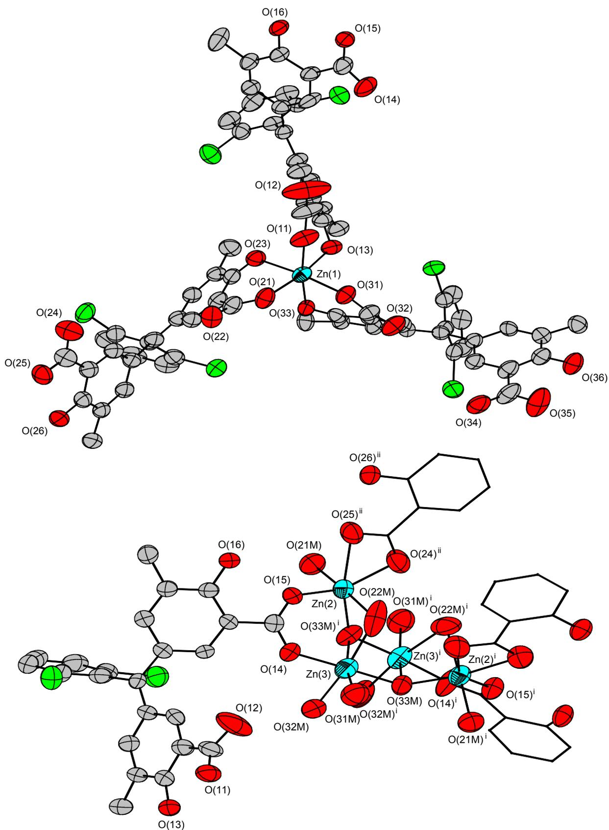
Fig. S8. Coordination environment of Zn(1) (*top*), Zn(2) and Zn(3) (*bottom*) atoms in **2**. Cryallographically independent atoms and coordination spheres of metal cations are shown in ellipsoids (50% probability). Hydrogen atoms are omitted. Symmetry transformations used to generate equivalent atoms: i)  $-x + 3/2, y, -z + 1$ ; ii)  $x + 1/2, -y + 1/2, -z + 1$ .
