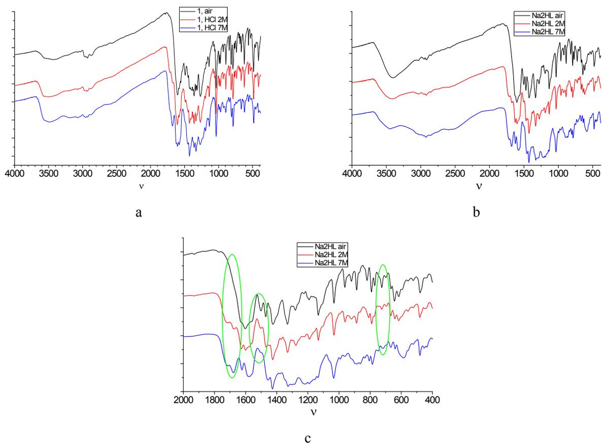
Fig. S13. IR spectra for (a) **1** and (b) Chromeazurol B exposed to air (black), under 2M HCl vapors (red), under 7M HCl vapors (blue), (c) Chromeazurol B in the range 400-2000  $\text{cm}^{-1}$ .
