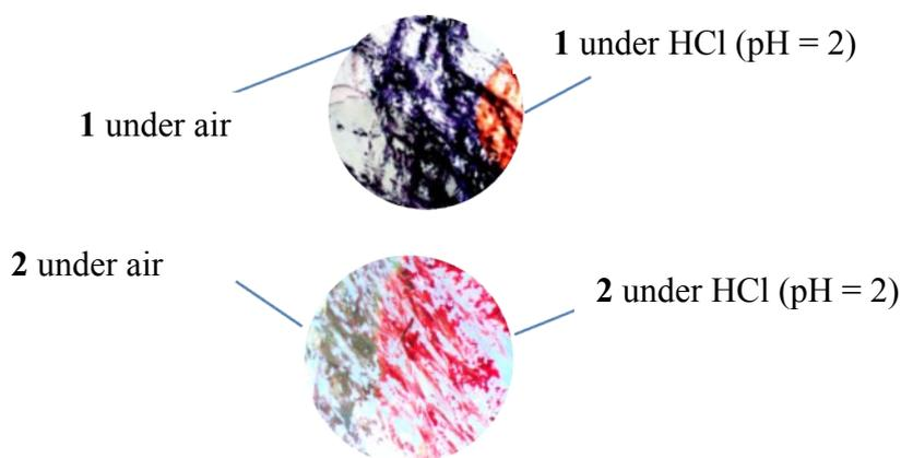
Fig. S9. View of halochromism in solutions for thin layer of **1** (top) and **2** (bottom) under different conditions.
