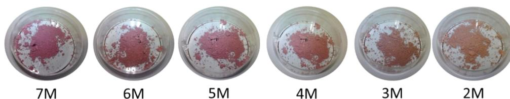
Fig. S10. Photographs of **1**@BaSO<sub>4</sub> in vapors of the hydrochloric acid of different concentration.
