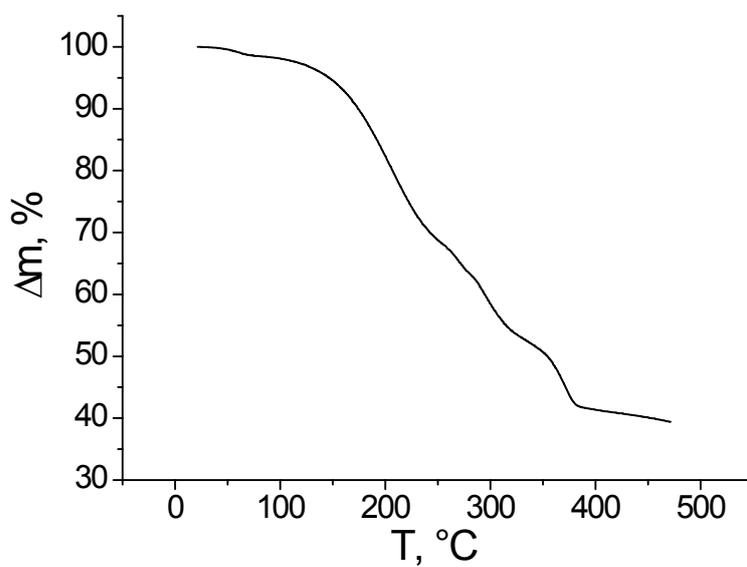
Figure S3. Thermogravimetric analysis of **1**.
