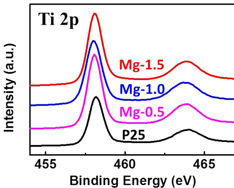
**Fig. S4** XPS spectra of the controllable reduced titania and pristine P25 nanoparticles.
