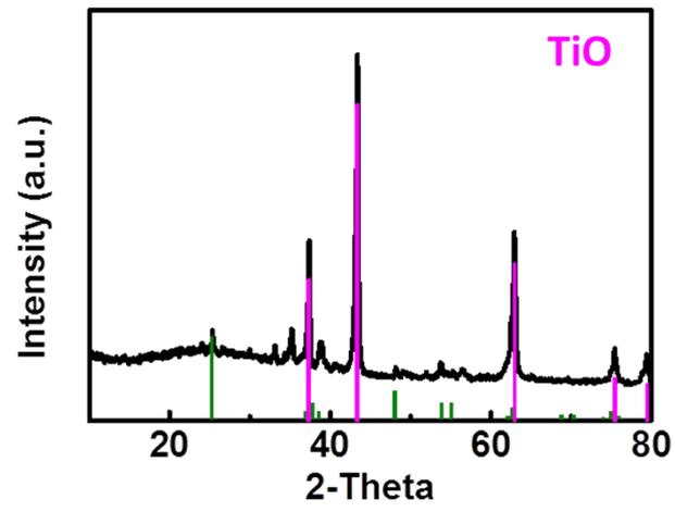
**Fig. S2** XRD patterns obtained black titania of Mg-2.0 reacted at 500 °C.
