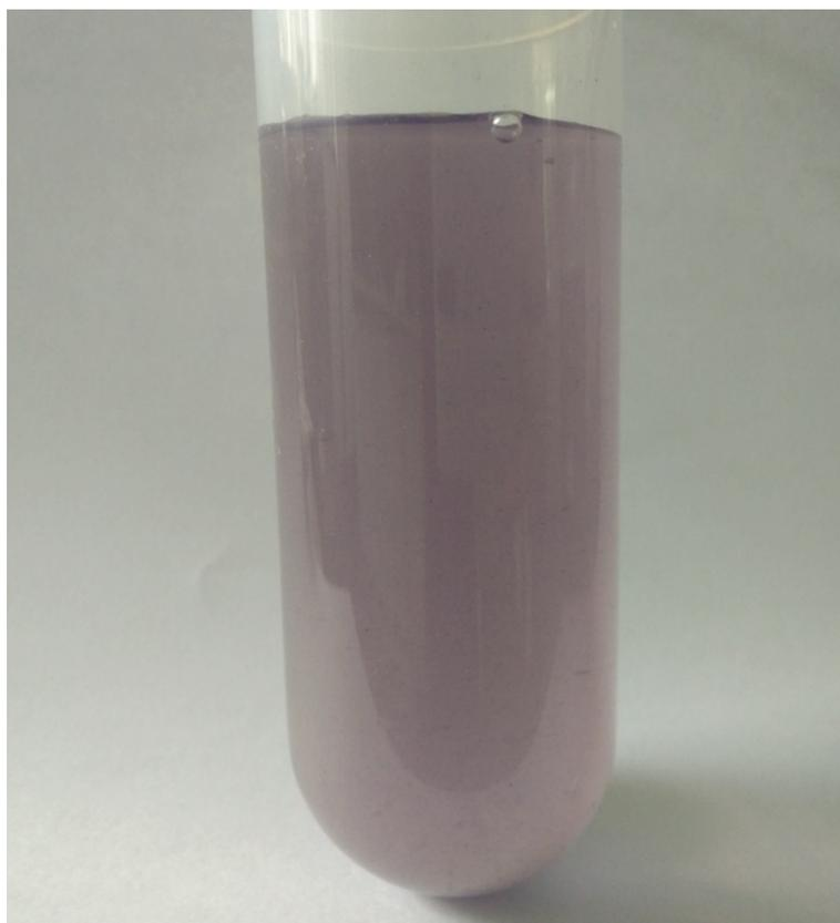
**Fig. S3** The purple solution consisting of  $\text{Ti}^{3+}$  obtained by Mg-2.0 reacted at 550 °C with the use of dilute HCl.
