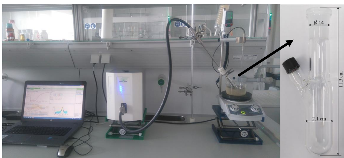
Figure 1. Hydrosilylation of alkynes with POSS 1 monitored by in situ FT-IR spectroscopy.
