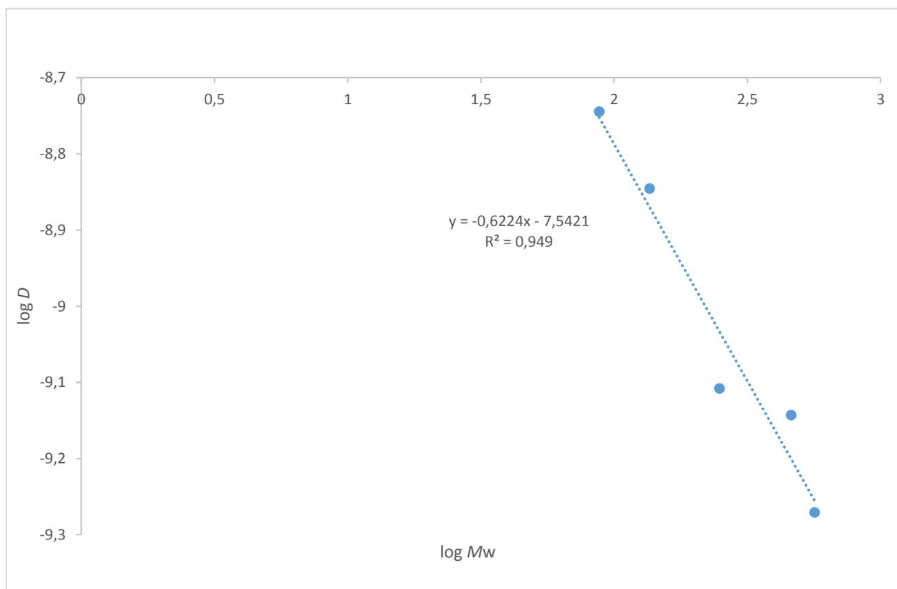
**Figure S18** Logarithmic diffusion coefficients  $D$  plotted against the logarithmic molecular weight of model compounds **11**, **17** and external standards 1,3,5-tris(trimethylsilylethynyl)-1,3,5-trimethyl-1,3,5-trisilacyclohexane,<sup>[S5]</sup>  $\text{Si}(\text{Me})_4$ <sup>[S6]</sup> and adamantane<sup>[S6]</sup>.
