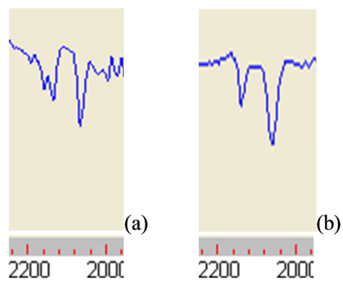
Figure S10. ATR-FTIR spectra for (a) a freshly prepared solution (5 min from mixing, 20 °C) of fac -[Ru 2 (CO) 6 Cl 4 ], 1 , CORM2, (6.8 mg) in 1 mL CH 3 OH+50 μL DMSO; and (b) same as (a) but after 90 min from mixing. The IR region is between 1960 and 2240 cm -1 for both spectra.
