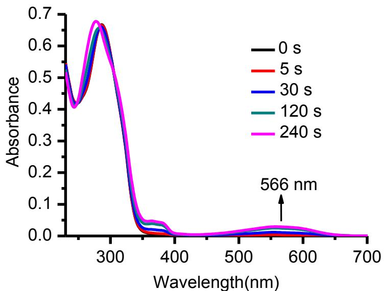
**Fig. S4** The UV-vis spectral changes of L1o ( $1 \times 10^{-5}$  M) in toluene upon irradiation at 312 nm.
