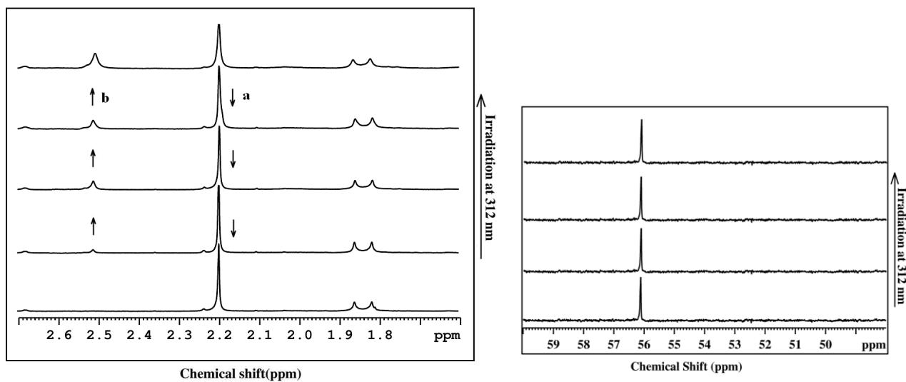
**Fig. S8** The  $^1\text{H}$  NMR (left) and  $^{31}\text{P}$  NMR (right) spectral changes of **1o** in  $\text{C}_6\text{D}_6$  upon irradiation with UV light at 312 nm.
