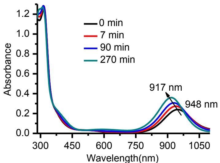
**Fig. S6** The UV-vis-NIR spectral changes of [3oo]<sup>-</sup> (1×10<sup>-5</sup> M) in toluene upon irradiation with UV light at 312 nm.
