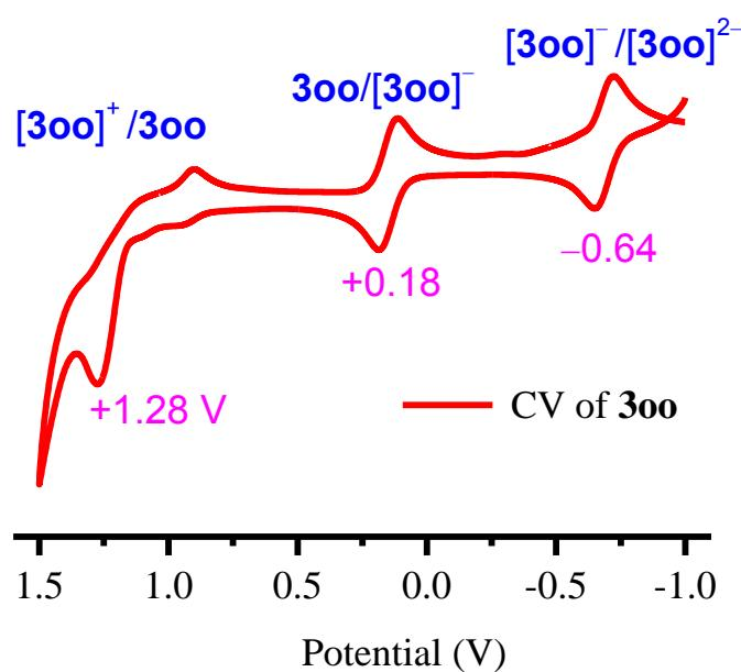
**Fig. S3** Plots of cyclic voltammogram of **3oo** in 0.1 M ( $\text{Bu}_4\text{N}^+$ ) $(\text{PF}_6^-)$  dichloromethane.
