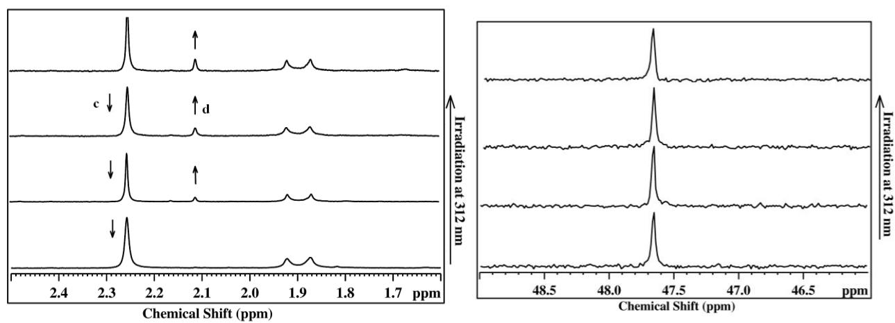
**Fig. S9** The <sup>1</sup>H NMR (left) and <sup>31</sup>P NMR (right) spectral changes of **2o** in C<sub>6</sub>D<sub>6</sub> upon irradiation with UV at 312 nm.
