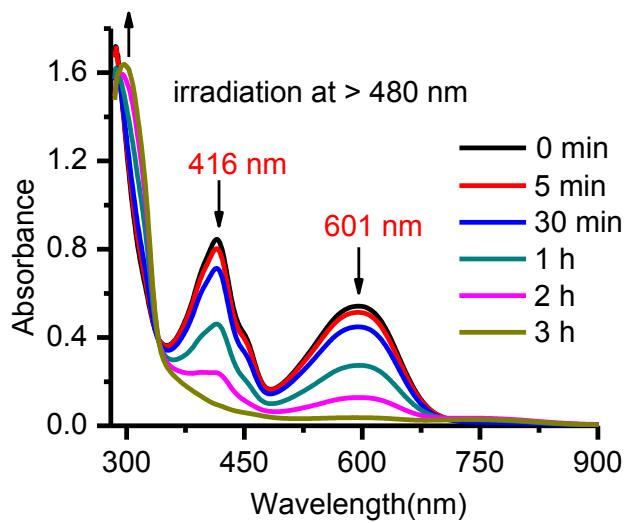
**Fig. S7** The UV-vis spectral changes of  $[4\text{cc}]^{2-}$  ( $1 \times 10^{-5} \text{ M}$ ) in DMSO upon irradiation with visible light at  $> 480 \text{ nm}$ .
