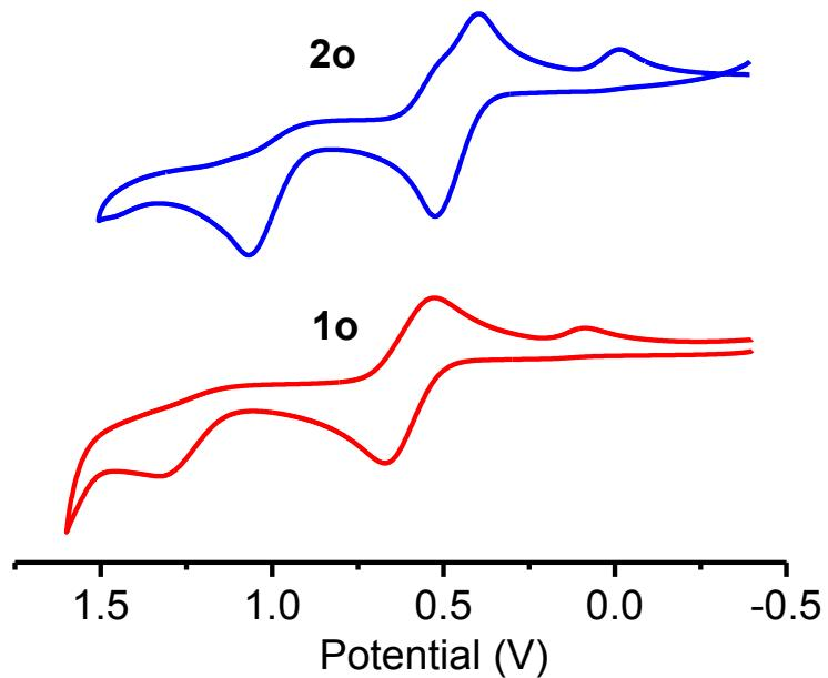
**Fig. S2** Plots of cyclic voltammogram of **1o** and **2o** in 0.1 M (Bu<sub>4</sub>N)(PF<sub>6</sub>) dichloromethane.
