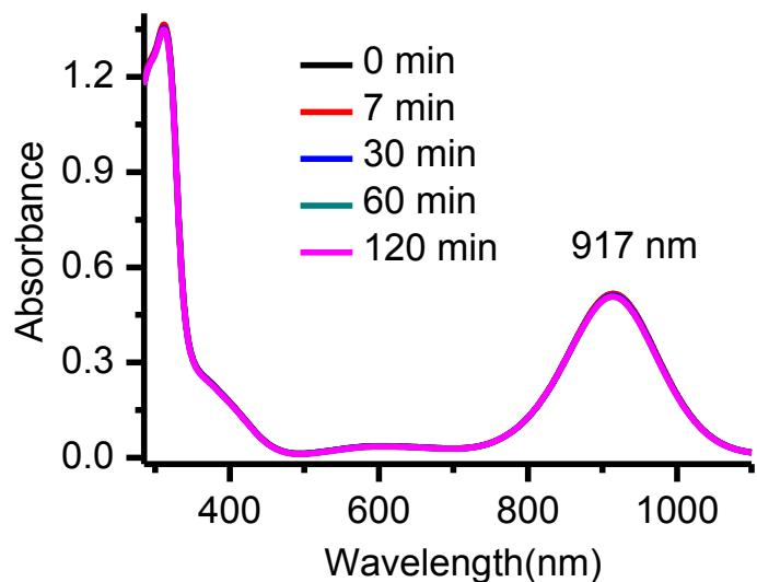
**Fig. S5** The UV-vis-NIR spectral changes of **3oo** (1×10<sup>-5</sup> M) in toluene upon irradiation with UV light at 312 nm.
