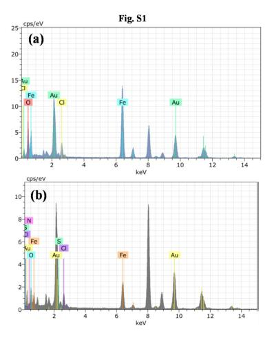
Fig. S1 the EDS spectra for  $Fe_3O_4/Au$  core/satellite nanoparticles and streptavidin immobilized  $Fe_3O_4/Au$  core/satellite nanoparticles.
