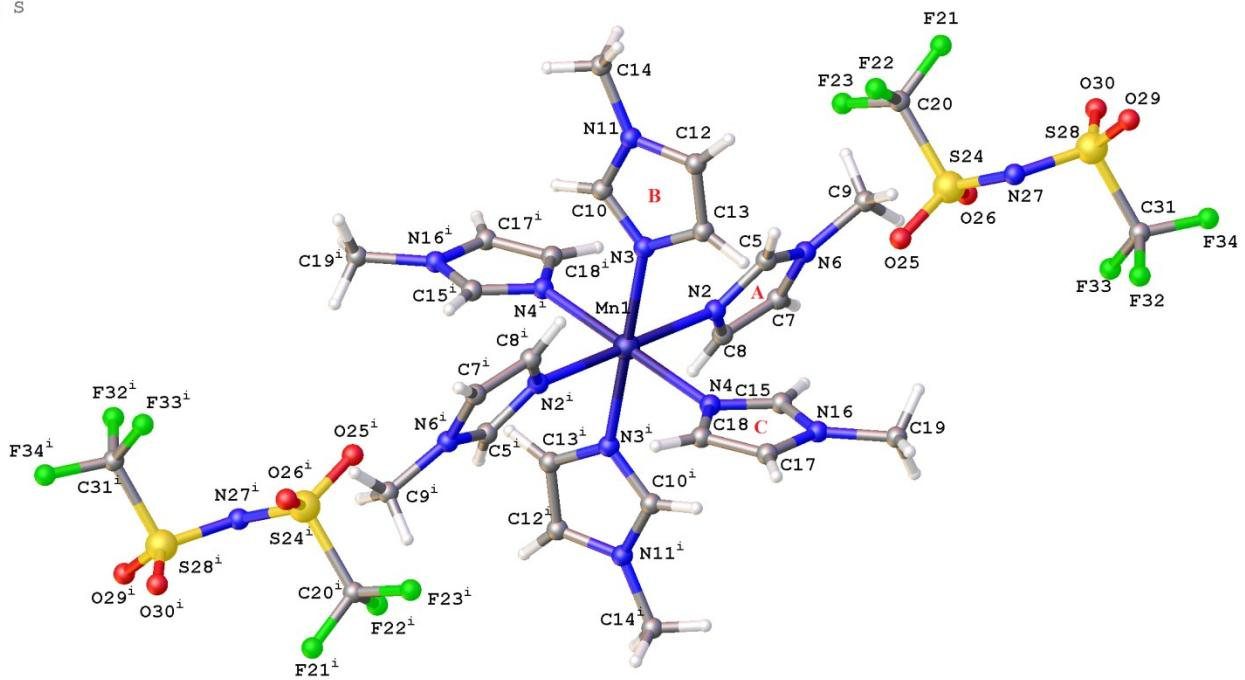
**Figure S2:** View of the crystal structure of  $[\text{Mn}(\text{MeIm})_6][\text{Tf}_2\text{N}]_2$ . Symmetry code: (i)  $1-x, 1-y, -z$ .
