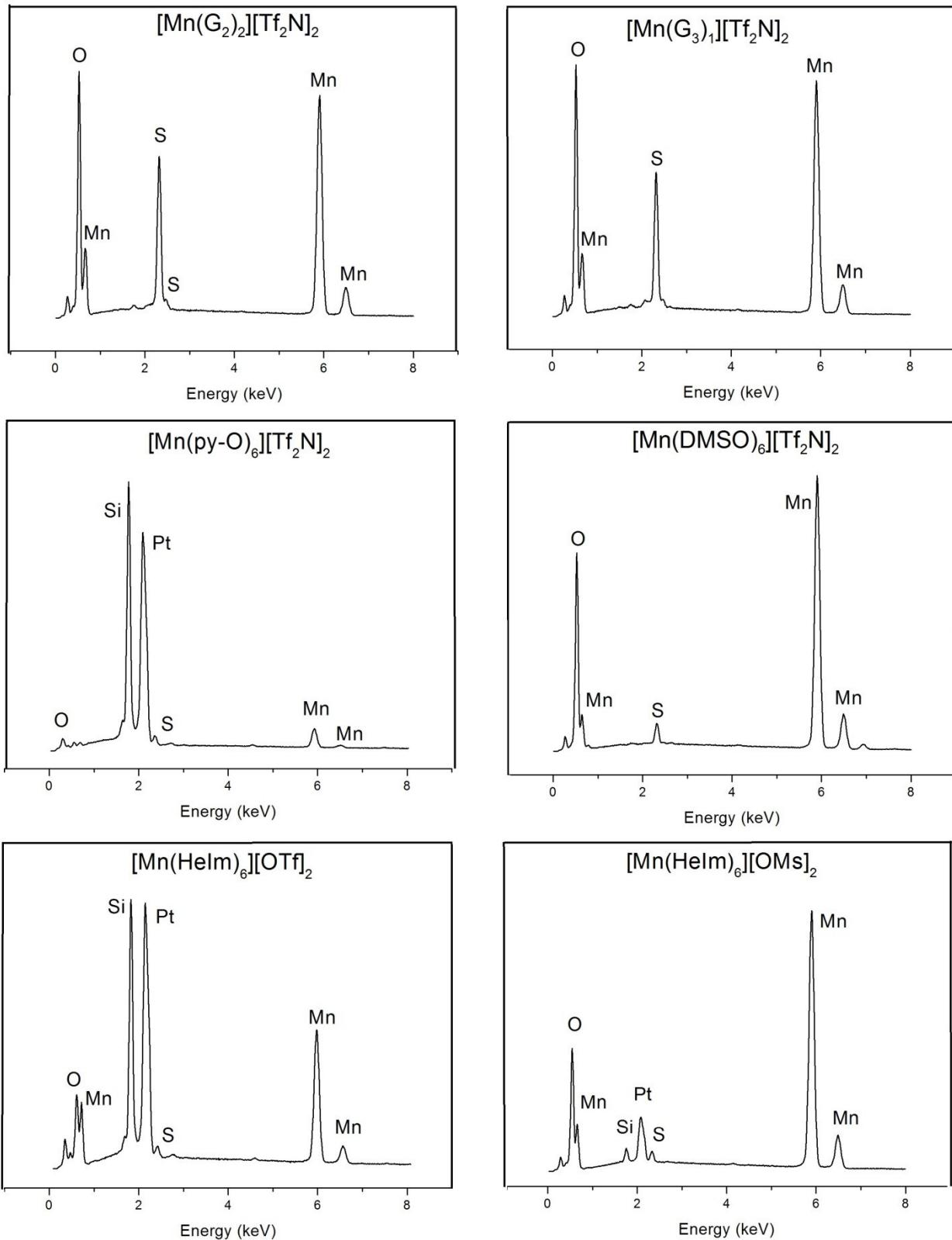
**Figure S8:** EDX spectra of the deposits obtained by electrodeposition from [Mn(DMSO)<sub>6</sub>][Tf<sub>2</sub>N]<sub>2</sub>, [Mn(G<sub>2</sub>)<sub>2</sub>][Tf<sub>2</sub>N]<sub>2</sub>, [Mn(G<sub>3</sub>)<sub>1</sub>][Tf<sub>2</sub>N]<sub>2</sub> and [Mn(py-O)<sub>6</sub>][Tf<sub>2</sub>N]<sub>2</sub>.
