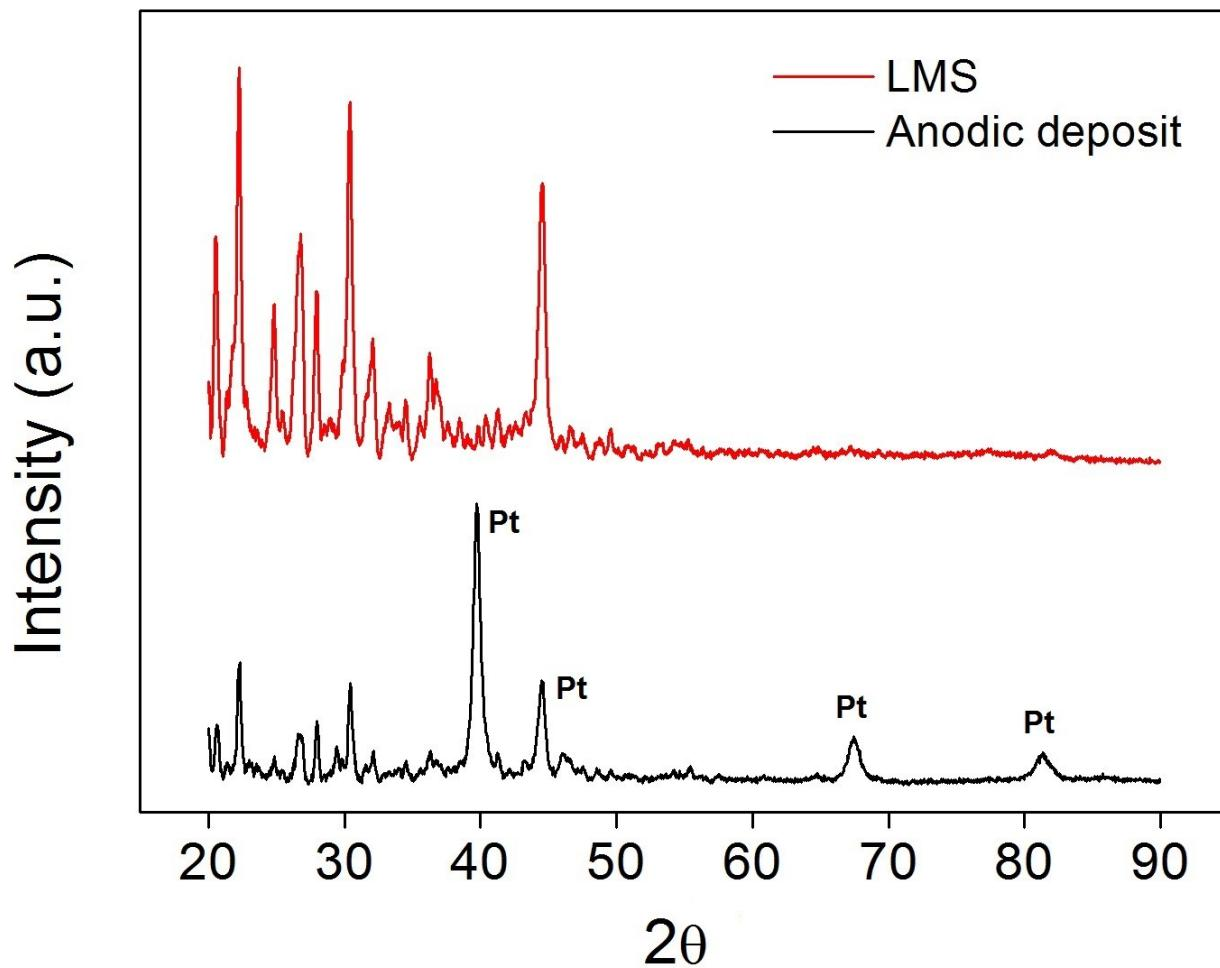
**Figure S5:** Grazing incidence X-Ray Diffraction pattern from the anodic deposit formed at +1.2 V vs Fc<sup>+</sup>/Fc in [Mn(py-O)<sub>6</sub>][Tf<sub>2</sub>N]<sub>2</sub> compared to that of pure [Mn(py-O)<sub>6</sub>][Tf<sub>2</sub>N]<sub>2</sub>.
