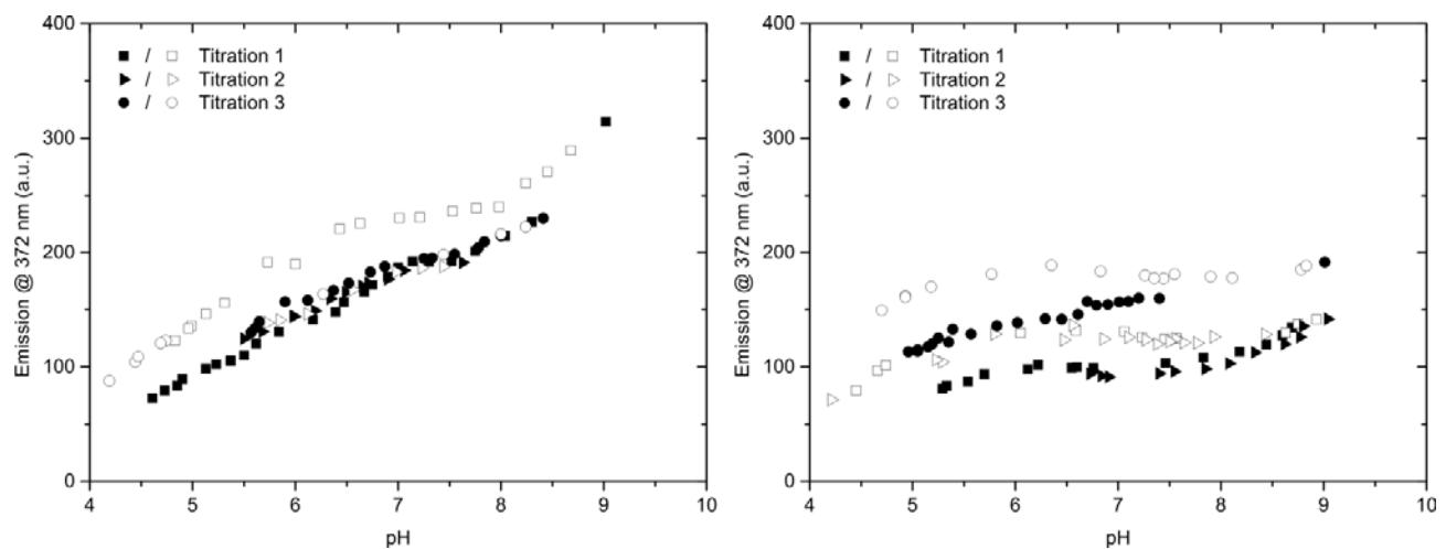
**Figure S3.** Fluorescence emission of AvD5-AP3 at 372 nm in dependence of pH in the absence (left) or in the presence (right) of 6 mM Mg(II). Solid and open data points represent measurements in opposite pH directions, i.e. increasing and decreasing, respectively.
