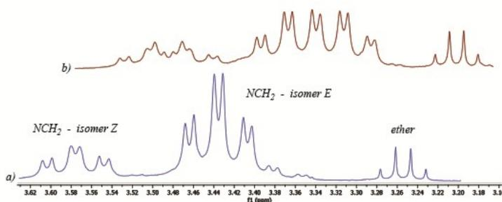
**Figure S4.** (a) Selected sections of  $^1\text{H}$  NMR (500 MHz,  $\text{C}_6\text{D}_6$ ) spectrum of complex **4**, signals assigned to the  $-\text{NCH}_2$  proton of *Z* and *E* isomers; (b) the same sample after addition of *ca.* equimolar amount of chiral reagent **5** (brown top line).
