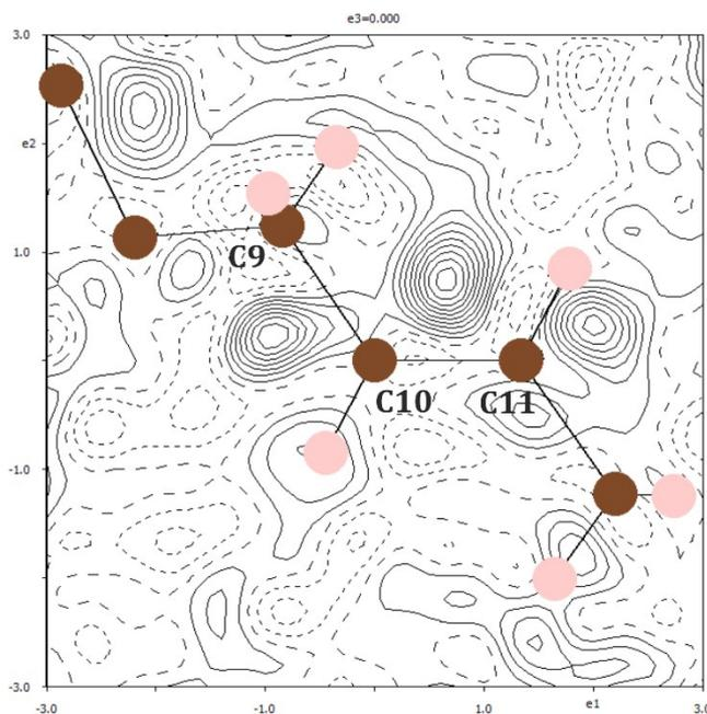
**Figure S2.** Fourier residual density map in the vicinity of the C10=C11 double bond in the crystal structure of complex **4**; the *Z* configuration is clearly visible (though the refinement was not possible). Largest residual density peak amounts to about  $0.5 \text{ e} \cdot \text{Å}^{-3}$ .
