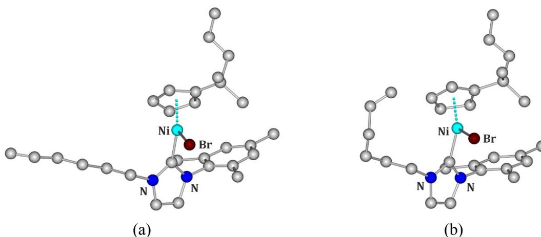
**Figure S1.** Molecular structure of two symmetry-independent species present in the crystal structure of **2** (space group:  $P2_1/n$ ,  $a = 20.554(2)$  Å,  $b = 11.3298(11)$  Å,  $c = 27.610(3)$  Å,  $\beta = 105.8624(19)^\circ$ ). Note that the structure is severely disordered and no full refinement is possible. Both symmetry-independent molecules (panels (a) and (b)) are shown separately with different orientations to indicate similarity with complex **1** (Figure 1a).
