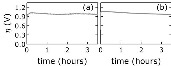
**Figure S8:** Constant current voltammograms of bare graphite electrodes in carbonate-containing (a) and virtually carbonate-free (b) electrolytes.
