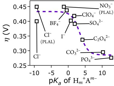
**Figure S10:** Overpotentials  $\eta$  of [NiFe]-LDH materials with different interlayer anions  $A^{m-}$  derived from constant current electrolysis at  $1 \text{ mA cm}^{-2}$  in virtually carbonate-free electrolyte as a function of anion basicity. Bare anion labels denote materials prepared by exchange from  $[\text{NiFe}](\text{NO}_3^-)$ -LDH.
