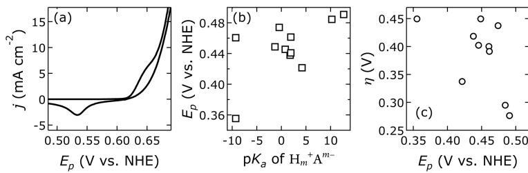
**Figure S11:** Magnified pre-water-oxidation-wave region of a representative cyclic voltammogram of [NiFe]-LDH nanosheets (a). Central polarization potential  $E_p$  of the reduction wave of [NiFe]-LDH nanosheets with different interlayer anions, collected in virtually carbonate-free electrolyte, as a function of anion basicity (b), and overpotential  $\eta$  as a function of  $E_p$  (c).
