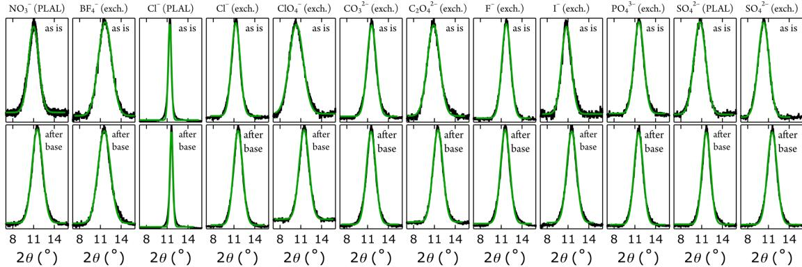
**Figure S6:** Gaussian fits (green) of the (001) peaks (black) of XRD data of [NiFe]-LDH nanosheets with different interlayer anions.
