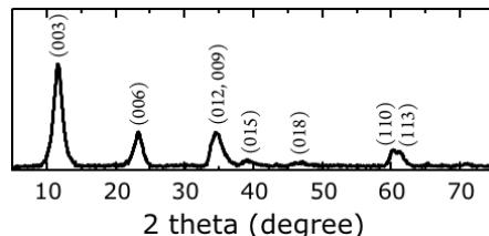
**Figure S5:** XRD data of [NiFe]-( $\text{CO}_3$ )-LDH nanosheets with indices of reflection.
