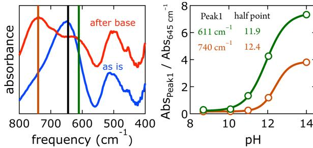
**Figure S12:** Left: Far-IR spectra of [NiFe]-(NO<sub>3</sub><sup>-</sup>)-LDH nanosheets as synthesized (as is) and after suspension in 1.0 M aqueous KOH in ambient air (after base). The vertical lines indicate the peaks that were analyzed. Right: Titration curves as a function of solution pH.
