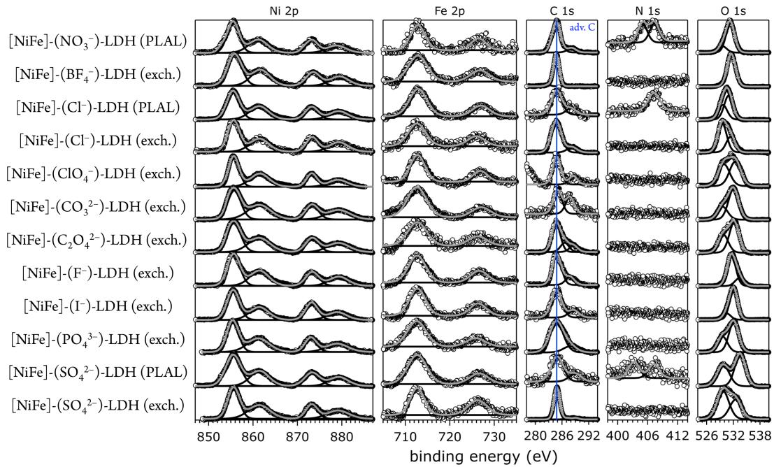
**Figure S1:** XPS data of [NiFe]-LDH nanosheets with different interlayer anions as synthesized in the Ni 2p, Fe 2p, C 1s, N 1s, and O 1s regions. The materials were prepared by pulsed-laser ablation in liquids (PLAL) or by anion exchange from [NiFe] $\cdot$ (NO<sub>3</sub><sup>-</sup>)-LDH (exch.). Open circles, data; black lines, peak fits; grey lines, envelopes. The blue line in the C 1s panel indicates the binding energy of adventitious carbon.
