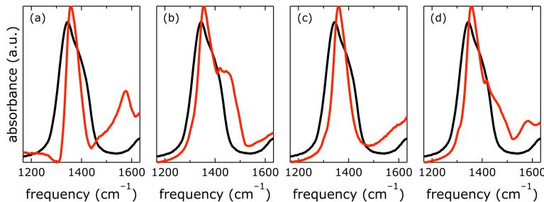
**Figure S7:** Infrared spectra of  $[\text{NiFe}]\text{-}(\text{NO}_3^-)\text{-LDH}$  nanosheets as synthesized (black) and after being suspended in 0.1 M aqueous KOH (red). The red spectra were taken using different suspension solution conditions: (a), in ambient air, no  $\text{Ba}(\text{OH})_2$ ; (b), in ambient air, with  $\text{Ba}(\text{OH})_2$ ; (c), in glove box, no  $\text{Ba}(\text{OH})_2$ ; (d), in glove box, with  $\text{Ba}(\text{OH})_2$ .
