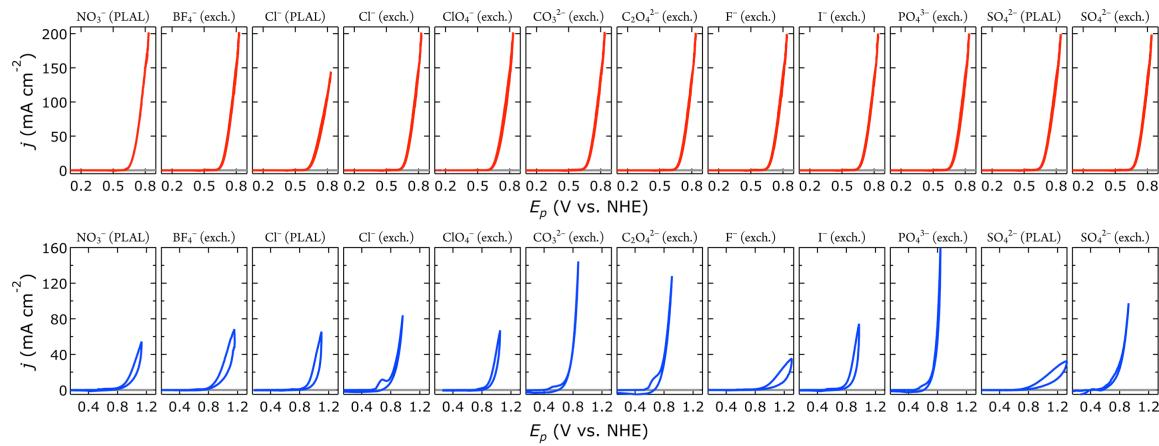
**Figure S9:** Cyclic voltammograms of [NiFe]-LDH materials with different interlayer anions in virtually carbonate-free electrolyte in a glove box (blue) and after suspension in 1.0 M aqueous KOH in ambient air (red). Cyclic voltammetry data of bare HOPG are shown in grey.
