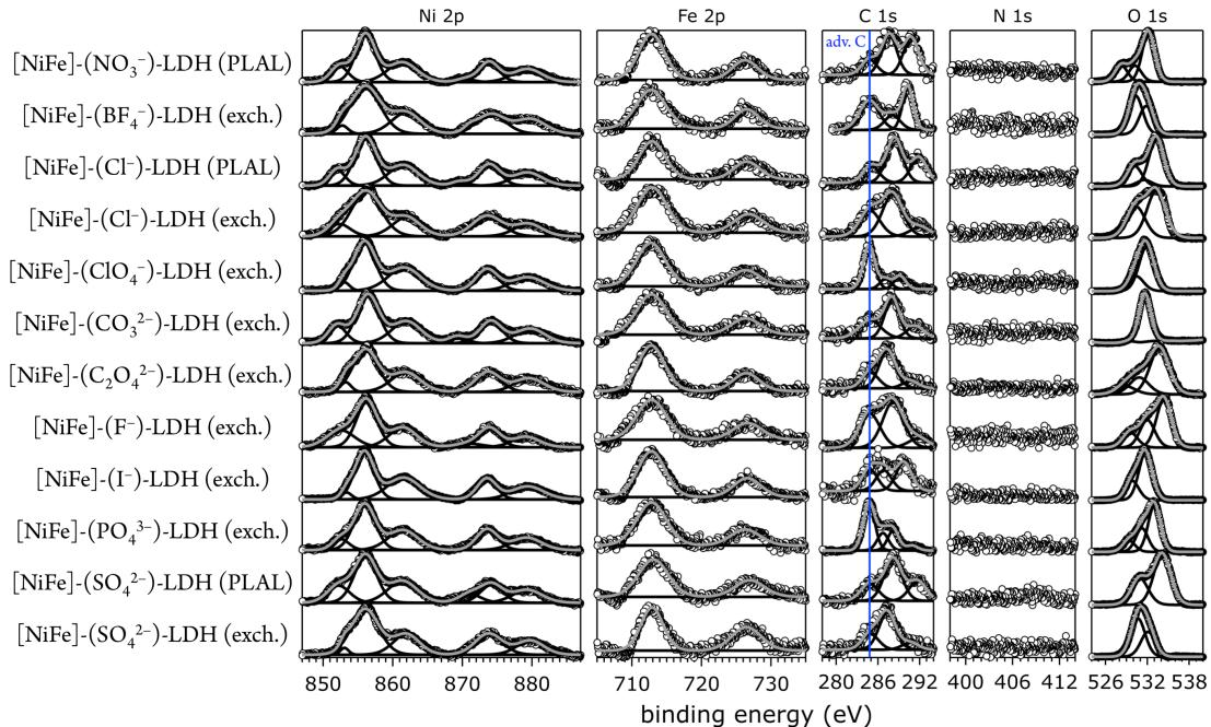
**Figure S2:** XPS data of [NiFe]-LDH nanosheets with different interlayer anions after suspension in 1.0 M aqueous KOH in ambient air in the Ni 2p, Fe 2p, C 1s, N 1s, and O 1s regions. The materials were prepared by pulsed-laser ablation in liquids (PLAL) or by anion exchange from [NiFe] $\cdot$ (NO<sub>3</sub><sup>-</sup>)-LDH (exch.). Open circles, data; black lines, peak fits; grey lines, envelopes. The blue line in the C 1s panel indicates the binding energy of adventitious carbon.
