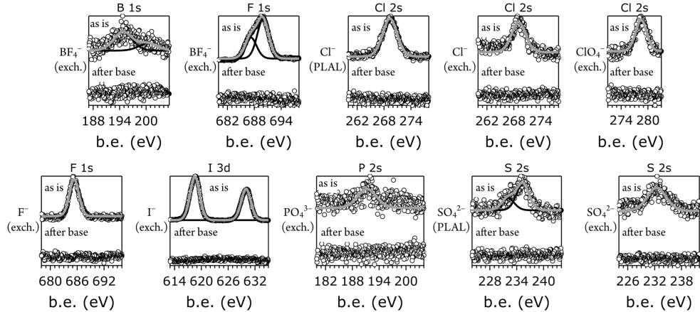
**Figure S3:** XPS data of [NiFe]-LDH nanosheets with different interlayer anions as synthesized (as is) and after suspension in 1.0 M aqueous KOH in ambient air (after base) in the B 1s, F 1s, Cl 2s, I 3d, P 2s, and S 2s regions, where applicable; b.e., binding energy. Open circles, data; black lines, peak fits; grey lines, envelopes.
