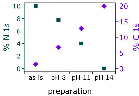
**Figure S4:** Quantification of the N 1s (teal) and C 1s (purple) regions of [NiFe]-( $\text{NO}_3^-$ )-LDH (as is) and exchanged in different pH aqueous KOH solutions in percent with respect to the total metal content.
