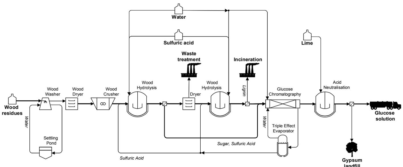
Fig. S1 Flowsheet for the production of *GLU* solution from wood residues.
