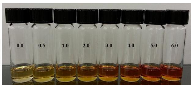
**Fig. 3** Photograph of the dissolved HMT-PMBI membranes in  $\text{DMSO-}d_6$  after 7 days in various NaOH concentrations (0.0 – 6.0 M) at 80 °C.
