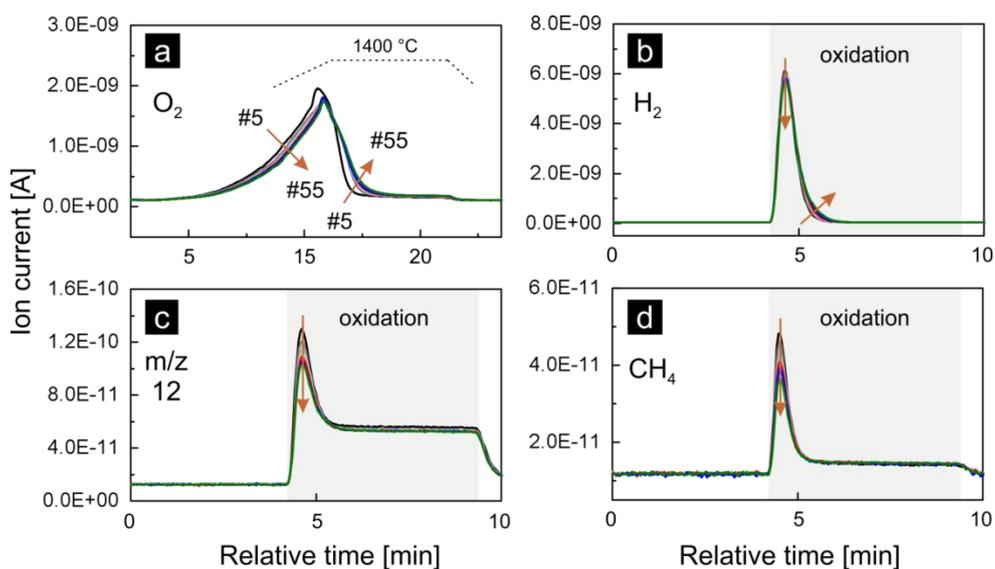
**Fig. S6** Comparison between cycles #5, #15, #25, #35, #45 and #55 during the long-term testing of rhodium-doped ceria at 1400|500 °C (results presented in Fig. 6): evolution of signals (a) oxygen, (b) hydrogen, (c)  $m/z = 12$  indicative of carbon monoxide, and (d) methane.
