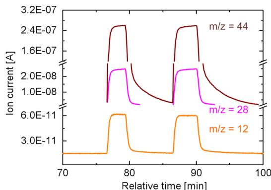
**Fig. S1** Ion current at  $m/z = 44$  ( $\text{CO}_2^+$ ), 28 ( $\text{CO}^+$ ) and 12 ( $\text{C}^+$ ) when carbon dioxide is introduced to the reactor at room temperature (no reaction, i.e.  $\text{CO}_2$  splitting, occurring). Due to fragmentation of  $\text{CO}_2$  to  $\text{CO}^+$  and  $\text{C}^+$  during ionization, the signals of  $m/z = 28$  and  $m/z = 12$  exhibit a step increase in the same manner as the signal of  $m/z = 44$ .
