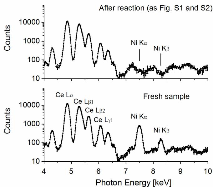
**Fig. S4** XRF results showing complete loss of nickel from nickel-doped ceria after 6 cycles at 1400|500 °C (Fig. S2) and the additional 11 cycles at 1500|500 °C (Fig. S3).
