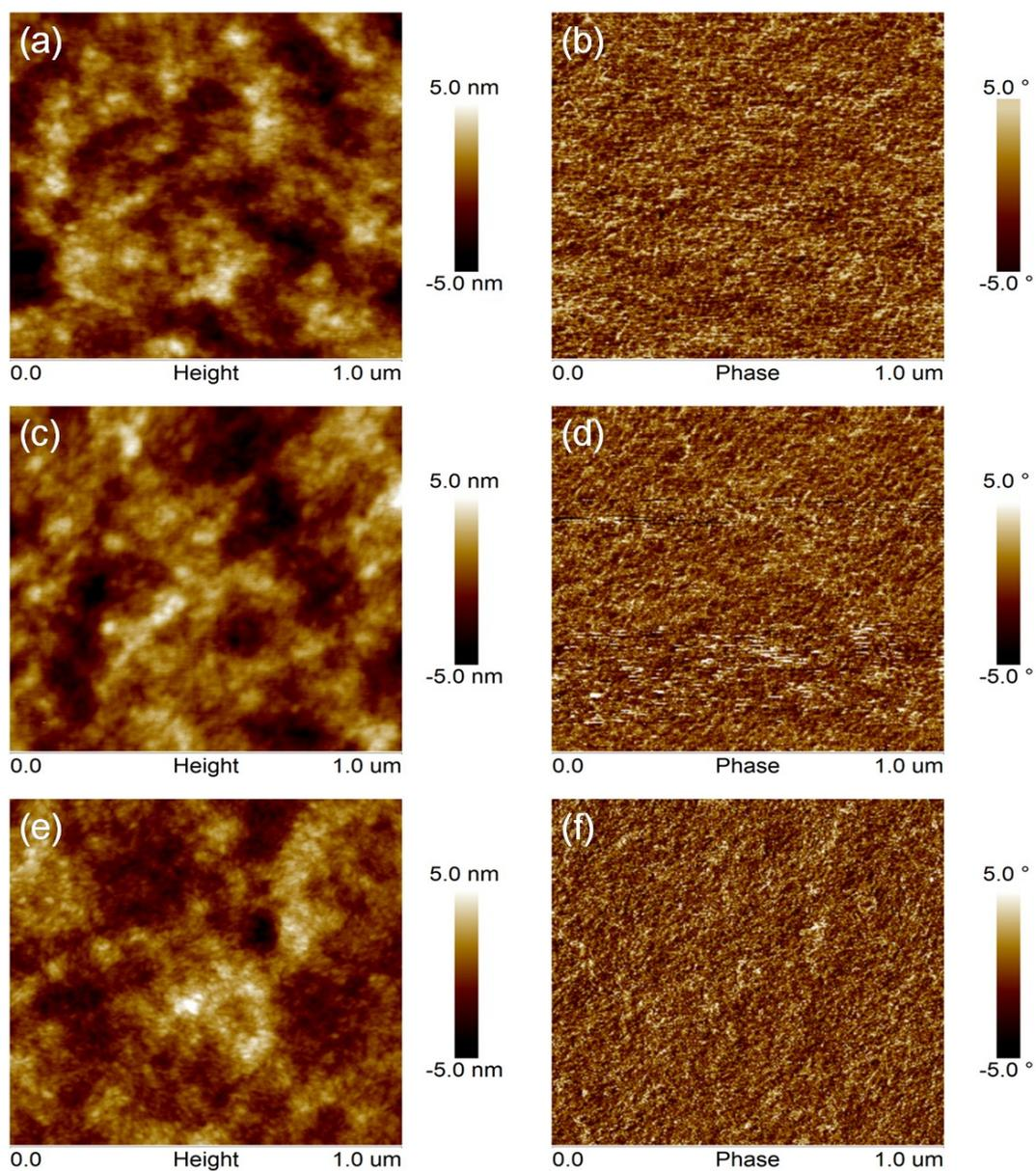
**Figure S32.** AFM height (left) and phase (right) images for the blend films. (a) and (b), PBDTTT-C-T:PC<sub>61</sub>BM blend; (c) and (d), PBDTTT-C-T:*e*-PPMF blend; (e) and (f), PBDTTT-C-T:*m*-PPMF blend.
