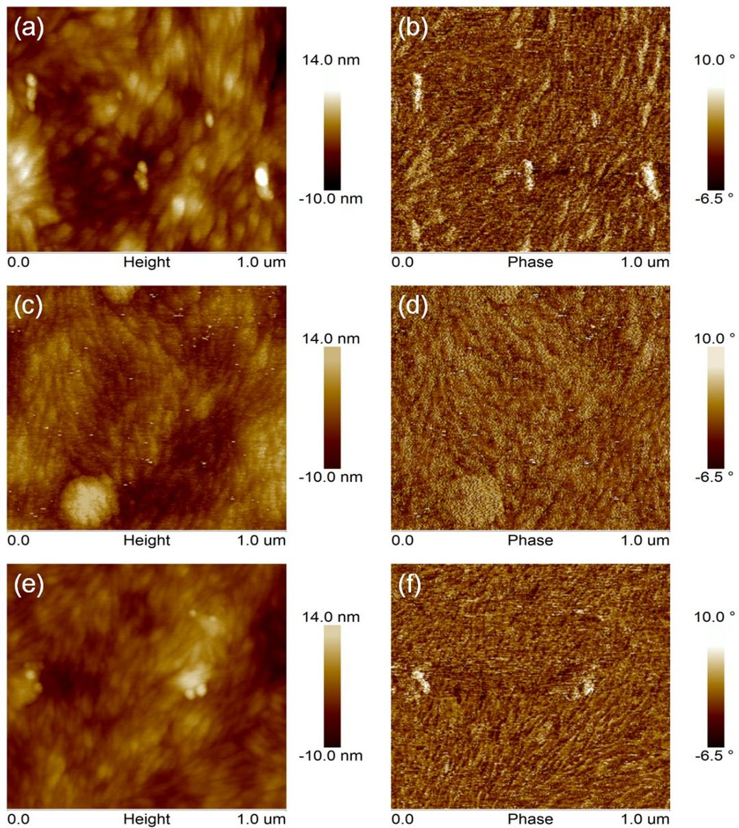
**Figure S31.** AFM height (left) and phase (right) images for the blend films. (a) and (b), PPDT2FBT:PC<sub>61</sub>BM blend; (c) and (d), PPDT2FBT:*e*-PPMF blend; (e) and (f), PPDT2FBT:*m*-PPMF blend.
