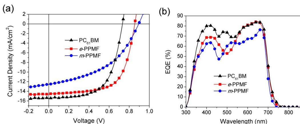
**Figure S27.**  $J-V$  curves (a) and EQE spectra (b) for PPDT2FBT:fullerene solar cells.
