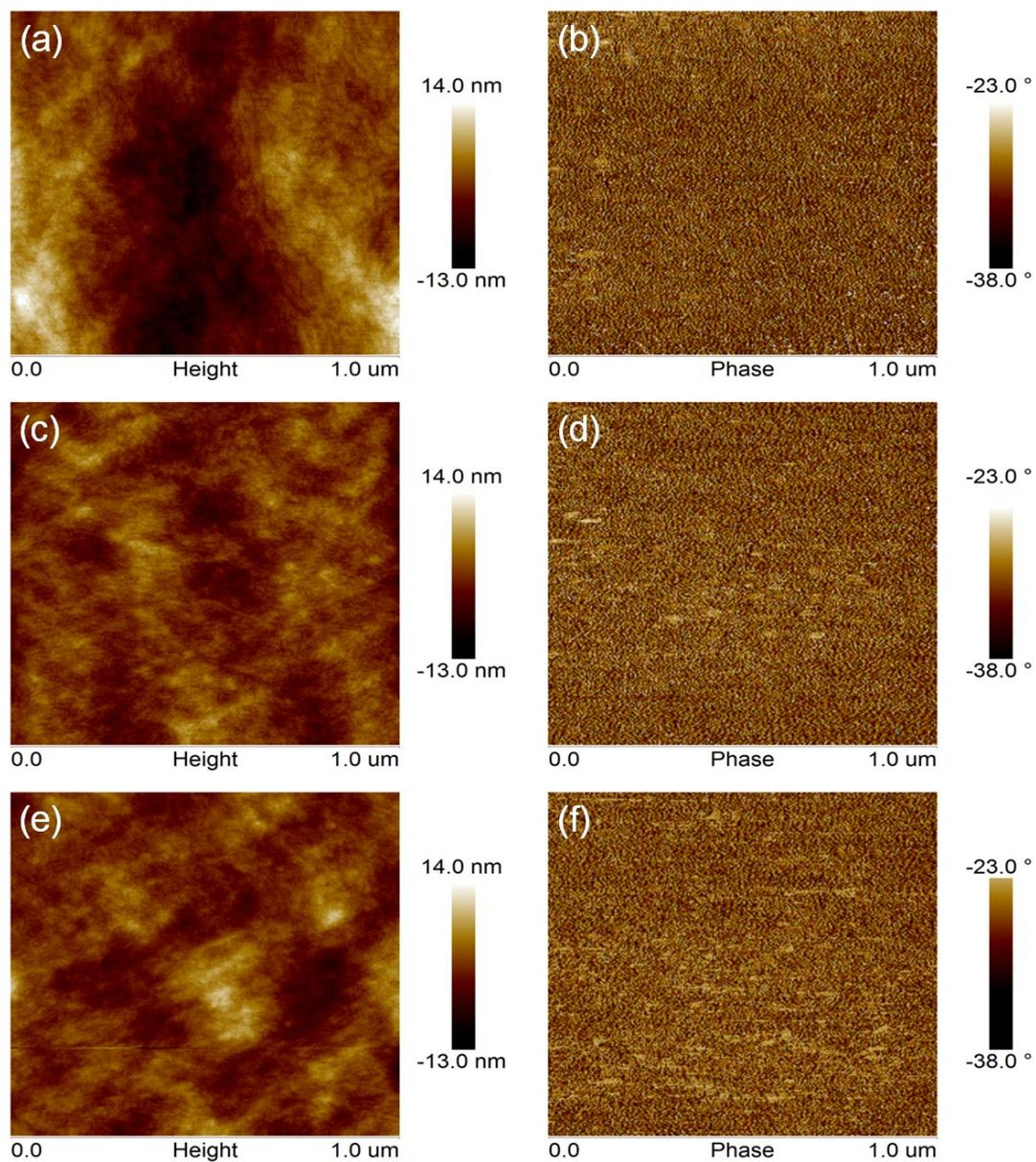
**Figure S30.** AFM height (left) and phase (right) images for the blend films. (a) and (b), P3HT:PC<sub>61</sub>BM blend; (c) and (d), P3HT:*e*-PPMF blend; (e) and (f), P3HT:*m*-PPMF blend.
