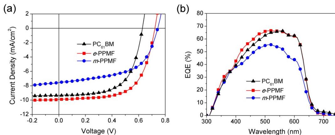
**Figure S26.** *J-V* curves (a) and EQE spectra (b) for P3HT:fullerene solar cells. The integrated photocurrent from EQE spectra for P3HT:PC<sub>61</sub>BM, P3HT:e-PPMF and P3HT:m-PPMF solar cells are 9.37, 9.53 and 7.52 mA/cm<sup>2</sup>, respectively.
