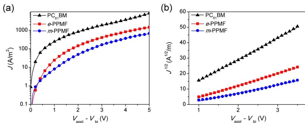
**Figure S29.**  $J$ - $V$  curves (a) and the corresponding  $J^{1/2}$ - $V$  plots (b) for electron-only devices based on P3HT:PC<sub>61</sub>BM, P3HT:e-PPMF and P3HT:m-PPMF blend films (in the dark). The thicknesses for the blend films are 247, 247 and 256 nm, respectively.  $\mu_e$  for PC<sub>61</sub>BM, e-PPMF and m-PPMF are  $7.49 \times 10^{-4}$ ,  $2.35 \times 10^{-4}$  and  $1.21 \times 10^{-4}$  cm<sup>2</sup> V<sup>-1</sup> s<sup>-1</sup>, respectively.
