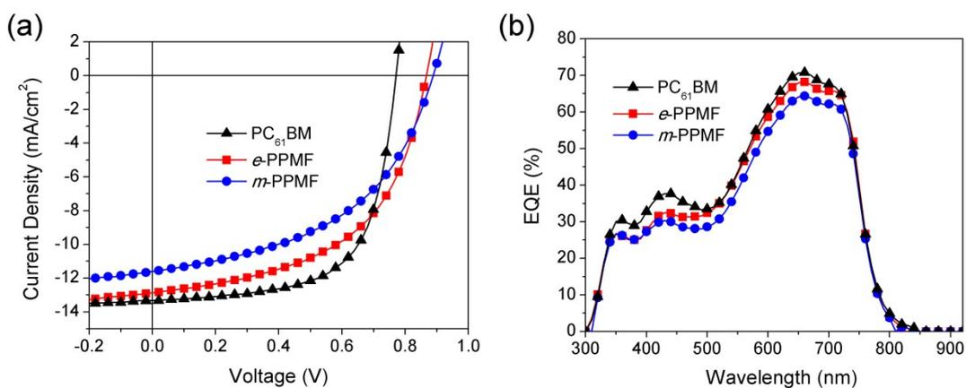
**Figure S28.**  $J-V$  curves (a) and EQE spectra (b) for PBDTTT-C-T:fullerene solar cells. The integrated photocurrent from EQE spectra for PBDTTT-C-T: $\text{PC}_{61}\text{BM}$ , PBDTTT-C-T: $e\text{-PPMF}$  and PBDTTT-C-T: $m\text{-PPMF}$  solar cells are 12.83, 12.30 and 11.44  $\text{mA}/\text{cm}^2$ , respectively.
