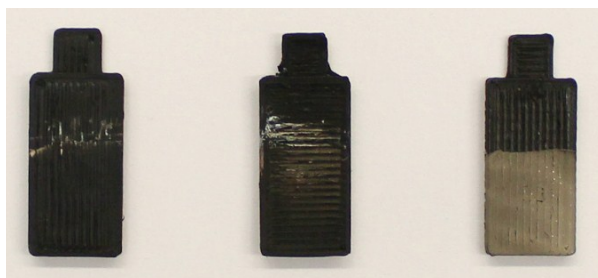
Figure S1. Electroplating comparison on 3D-printed electrodes. Left: Reprapper Conductive ABS, Middle: MatterHackers Conductive ABS, Right: Proto-Pasta conductive PLA .
