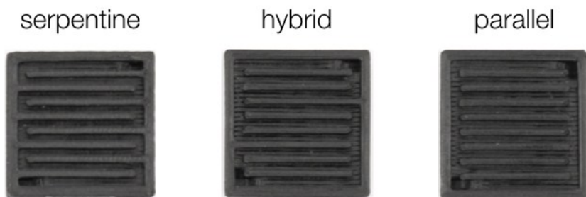
Figure S4. 3D-printed flow-field plates with three different flow-field patterns.
