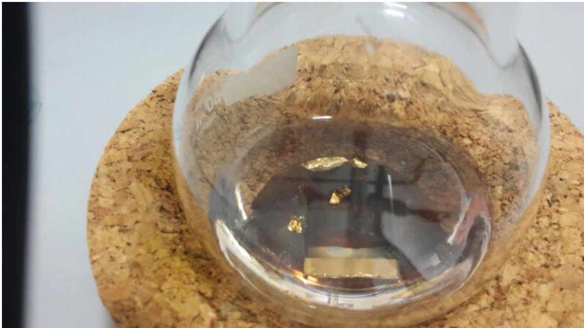
Figure S 2 Gold removal in chlorobenzene bath
