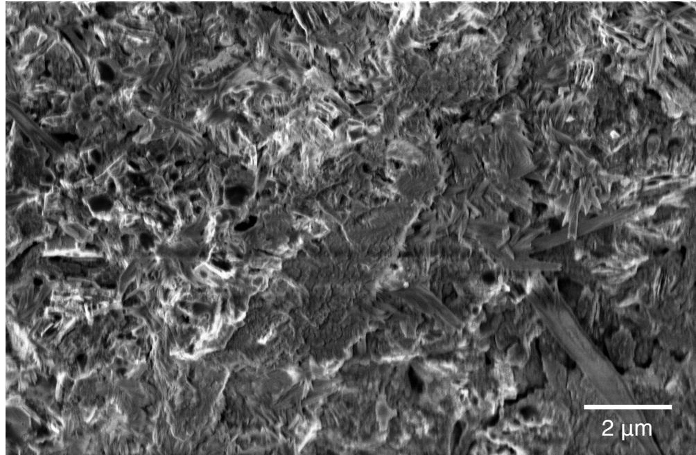
Figure S2: SEM images of the SrFeO<sub>3-δ</sub> sample.
