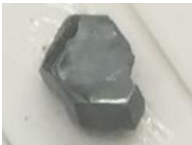
Figure S1 A recently took photograph of a single crystal. This crystal has been stored in air without encapsulation for more than 2 years. A photograph of this crystal was shown in our paper published about 2 year ago. 2
