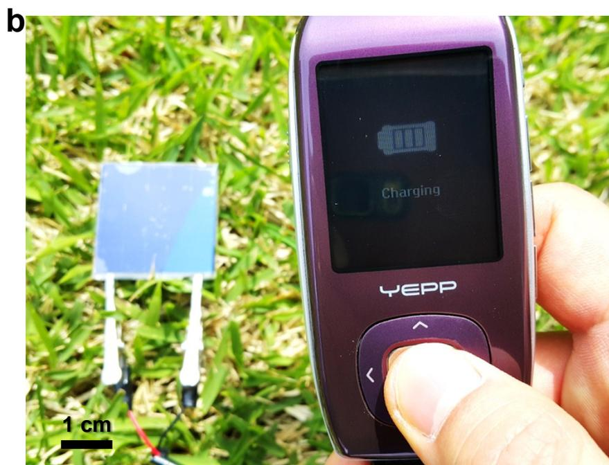
**Supplementary Movie S1.** Video clips showing portable electronics that are being charged by SiPV-LIB device under sunlight illumination. (a) smartphone. (b) MP3 player.
