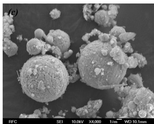
Fig. S1. Scanning electron microscopy (SEM) images of (a) Peerless iron, (b) iron sulfide, and (c) steel dust.
