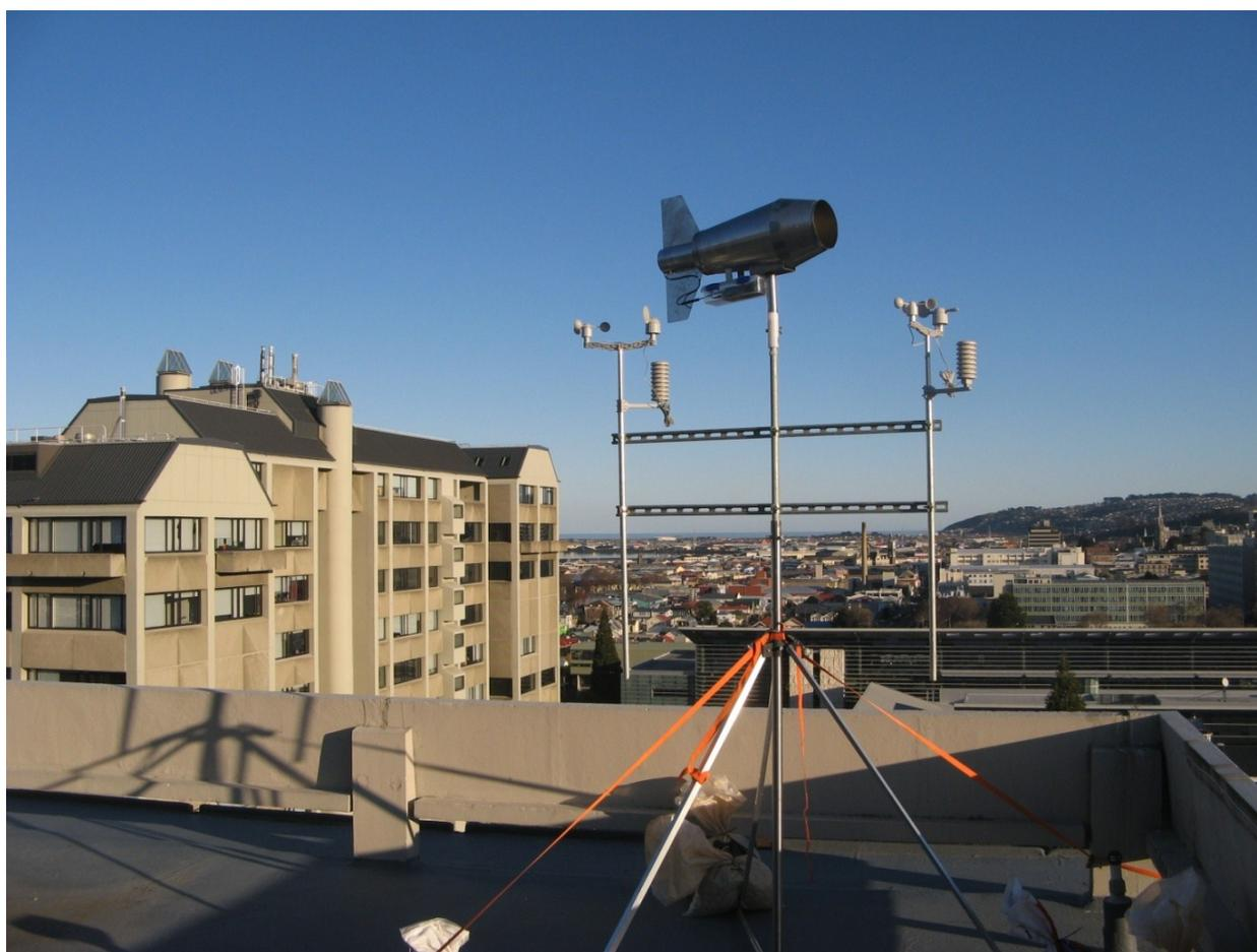
**Figure S1.** Flow-through sampler set up for field calibration on the Science II Building roof at the University of Otago, Dunedin, New Zealand.
