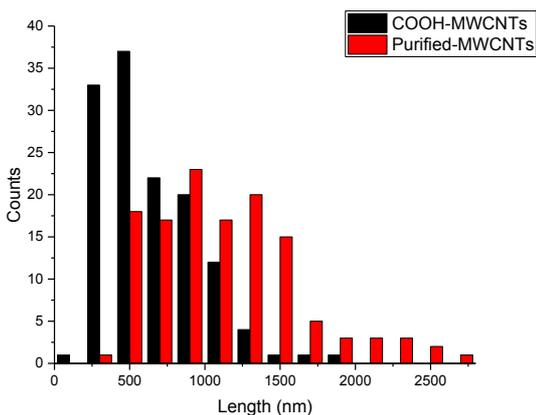
**Supplementary Figure S1.** The length distribution of COOH- and Purified-MWCNTs, obtained from over 100 SWCNTs imaged on independent positions across the specimen.
