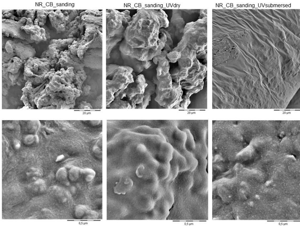
Figure SI\_11 Morphology of NR\_CB sanding fragments retrieved after immersion in M4 medium, in two magnifications, for the non-aged material, aged as dry powder, aged during submersion in M4 medium.
