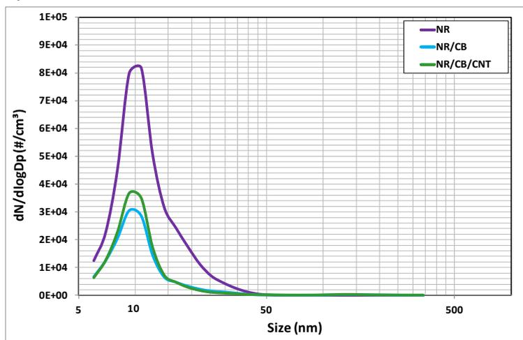
Figure SI\_10 Aerosol characterization during sanding. A) APS size distribution as determined in the sanding set-up; b) FMPS size distribution as determined in the sanding set-up.
