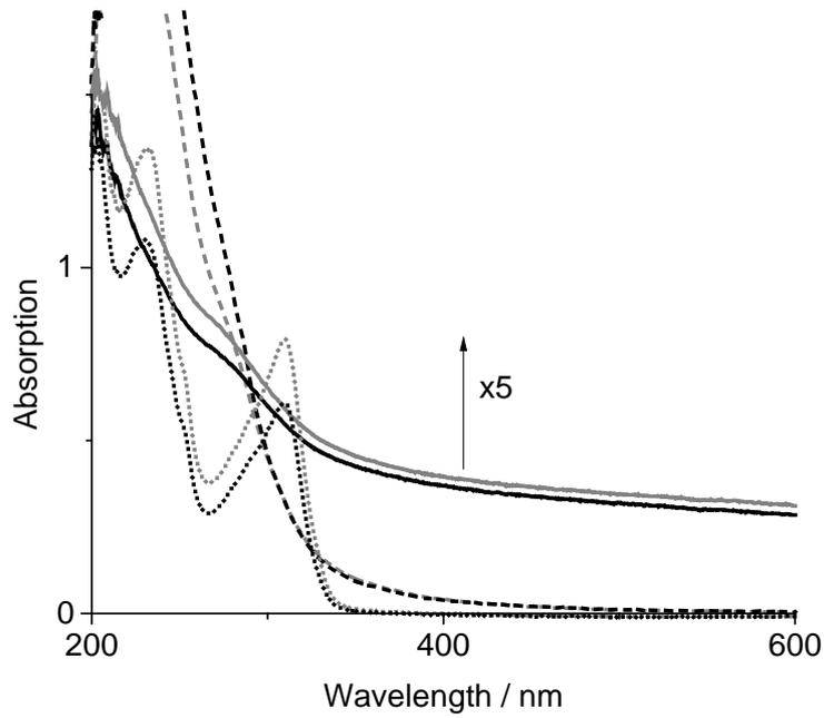
Figure SI\_13 Absorption of suspensions in M4 medium: NR\_CB (grey) and NR\_CB\_CNT (black). Sanding fragments (solid lines); Sanding fragments aged by UV light in M4 medium (dashed lines); Sanding Fragments aged dry by UV light, then suspended (dotted lines). All suspensions prepared at 10 g/L solid content, except the dry-aged materials (dotted lines) whose absorption saturated the detector at 10 g/L so that the data shown was obtained at concentrations reduced to 2 g/L.
