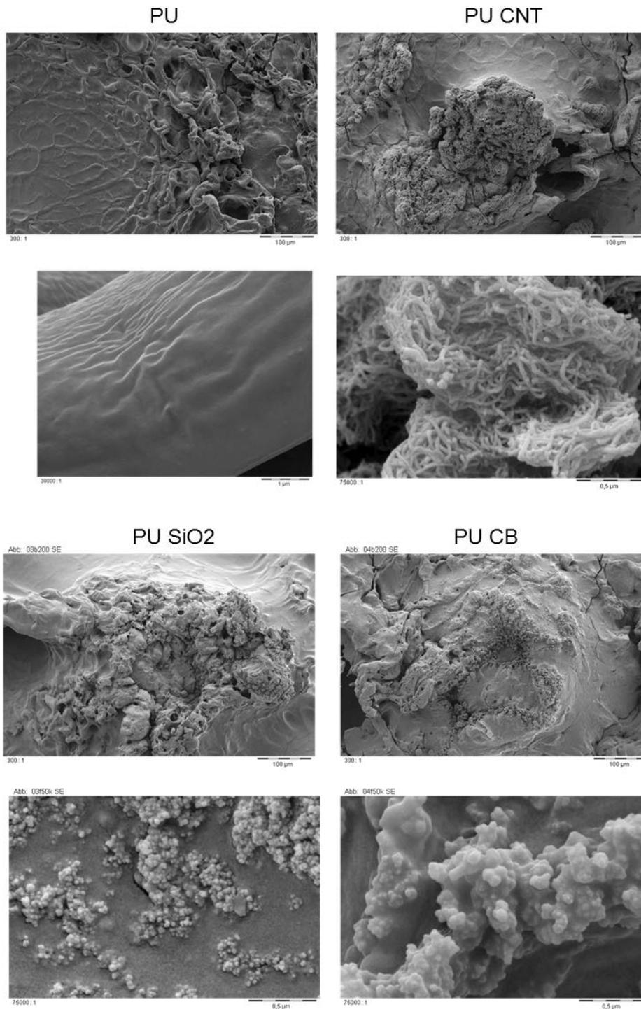
Figure SI\_4 Surface structure of PU and PU nanocomposites after UV and rain aging for 672h, by SEM.
