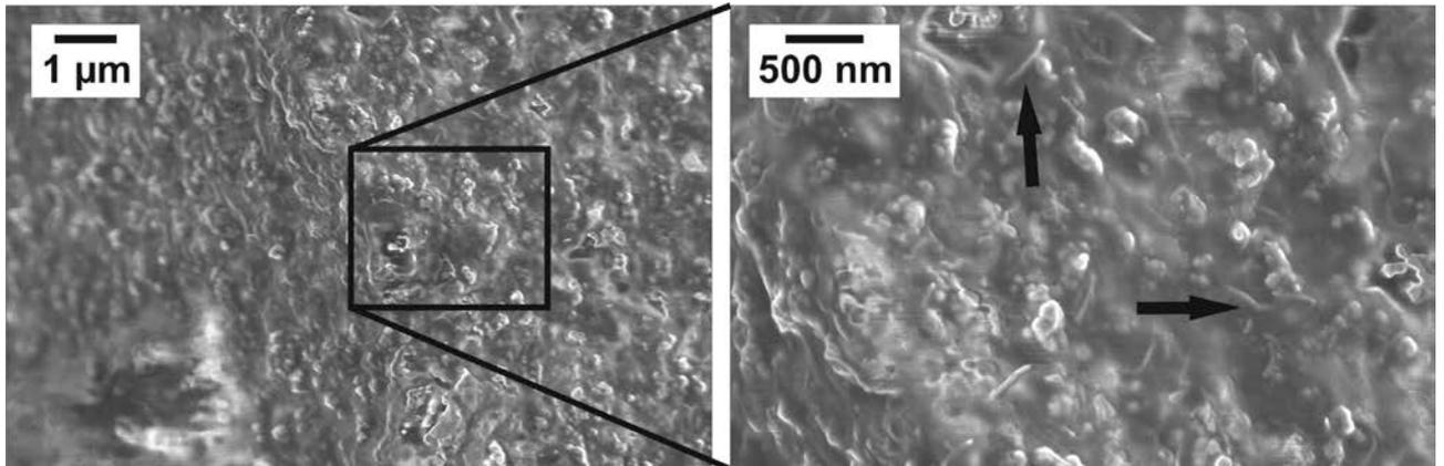
Figure SI\_7: SEM images in two different magnifications of as-prepared natural rubber + CB + CNT. The specimen was sliced out of the bulk sample and prepared on a SEM stub. Both the CB (cauliflower like structures) as well as the CNT (long tube-like structures) can be identified. The arrows point to CNT embedded in the sample.
