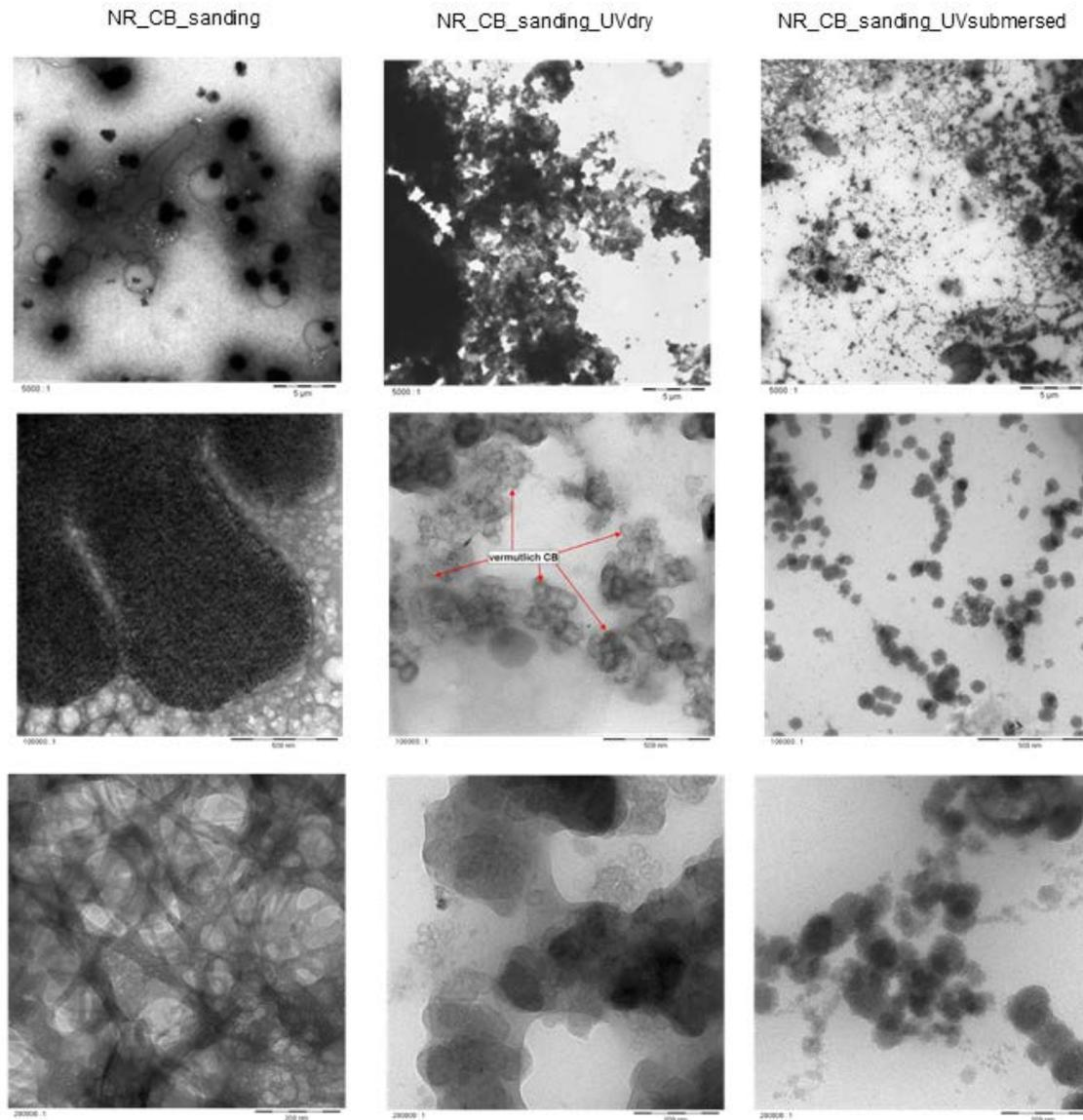
Figure SI\_14 Morphology of fragments released from NR\_CB sanding fragments after immersion in M4 medium and filtration with 5 $\mu$ m to remove the original sanding fragments. TEM scans in three magnifications (scale bars from top to bottom: 5 $\mu$ m, 500nm, 200nm), for the non-aged material, aged as dry powder, aged during submersion in M4 medium.
