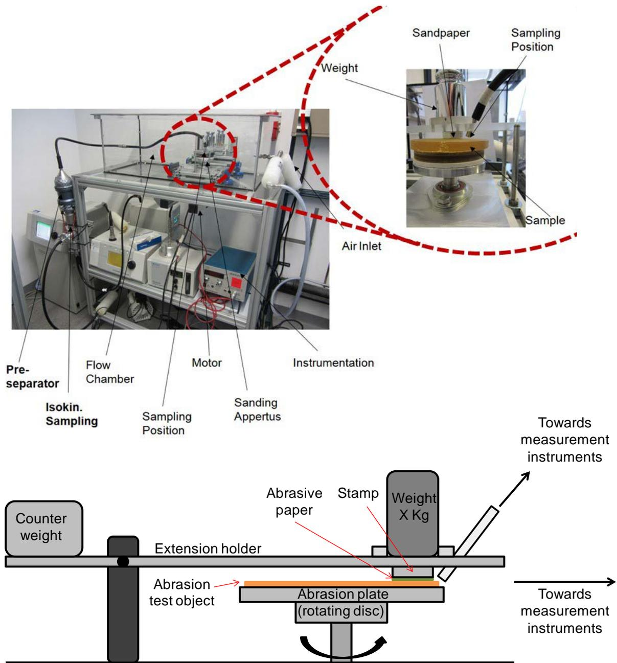
Figure SI\_8: Sanding test rig in the IUTA laboratory for NR, NR+CB, NR+CB+CNT samples. Sanding was conducted while this set-up was in a particle-free enclosure.
