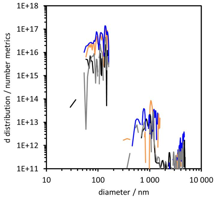
Figure SI\_2 Number metrics representation of the full size distributions of fragments sampled by immersion and sonication from the four PU materials after UV aging (with rain) for 535 MJ/m<sup>2</sup>. Measured by AUC, converted from mass metrics (Fig 8a) to number metrics. Neat TPU (orange); TPU\_CNT (black); TPU\_CB (grey); TPU\_SiO2 (blue);
