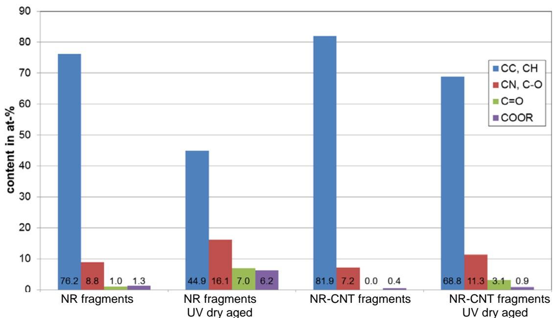
Figure SI\_12 Surface chemistry as determined by XPS photoelectron spectra with C(1s) line fit, comparing the sanding fragments before and after aging (UV 720h dry).
