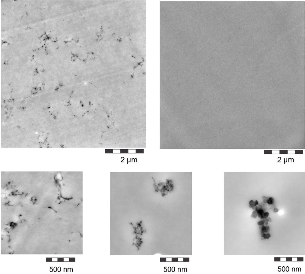
Figure SI\_1 TEM cross-sections of PU materials. A) PU\_CNT with larger field-of-view to reflect the degree of dispersion; b) PU reference; c) PU\_CNT at higher magnification; d) PU\_SiO2; e) PU\_CB.
