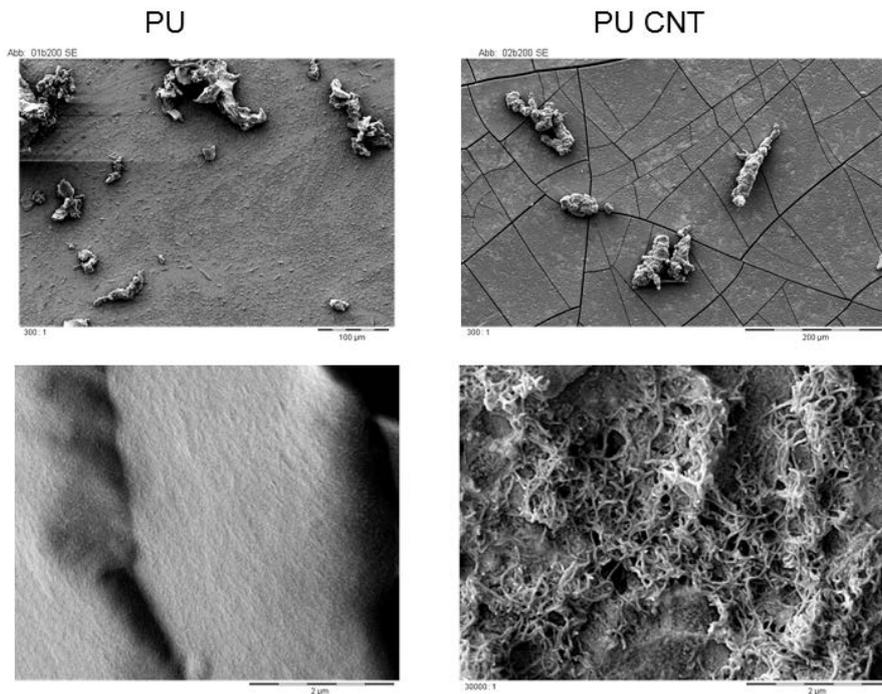
Figure SI\_5 Surface structure of PU and PU nanocomposites after UV (no rain) aging for 672h, by SEM.
