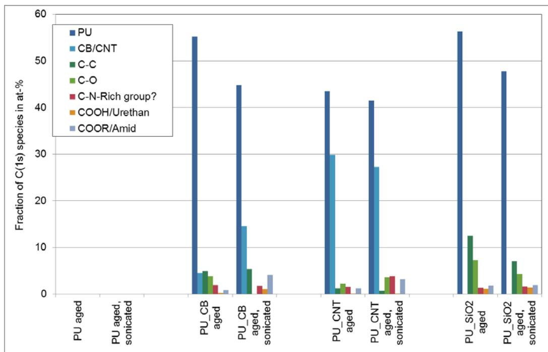
Figure SI\_6 Analysis of the specimen surface after aging, and after sonication sampling: C(1s) line fit results, using a non-aged neat PU as reference (dark blue), and separate positive control measurements of CB and CNT (light blue).
