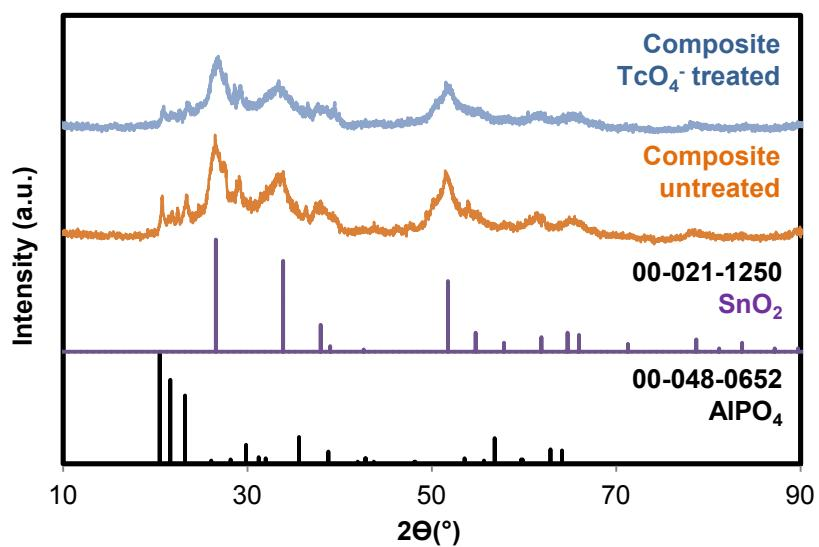
**Figure S2.** XRD patterns of the Sn-Al-PO<sub>4</sub> composite before and after exposure to an aqueous solution of TcO<sub>4</sub><sup>-</sup>
