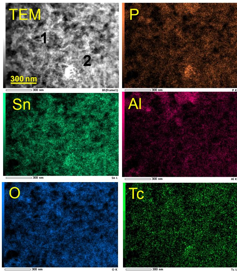
**Figure S3.** Representative elemental distribution in the amorphous matrix the 24 hour TcO<sub>4</sub><sup>-</sup> treated Sn-Al-PO<sub>4</sub> composite.
