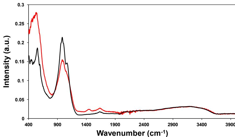
**Figure S1.** IR spectra of the Sn-Al-PO<sub>4</sub> composite (black trace) before TcO<sub>4</sub><sup>-</sup> exposure and (red trace) after 24 hour exposure to TcO<sub>4</sub><sup>-</sup>.
