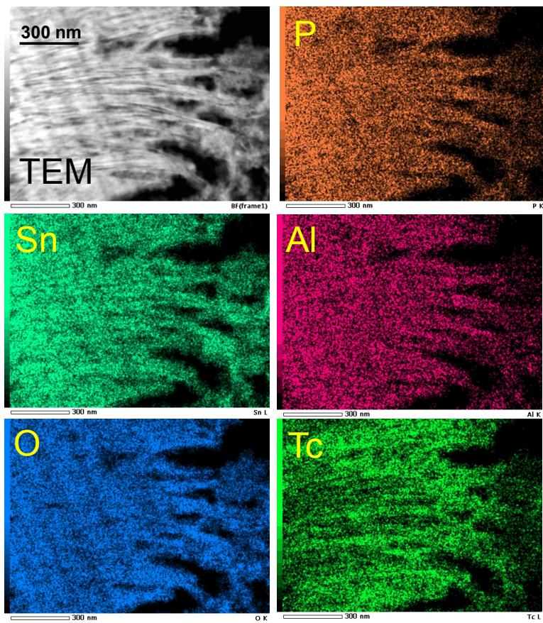
**Figure S4.** Representative elemental distribution in the crystalline fibers for the 24 hour  $\text{TcO}_4^-$  treated **Sn-Al-PO<sub>4</sub>** composite.
