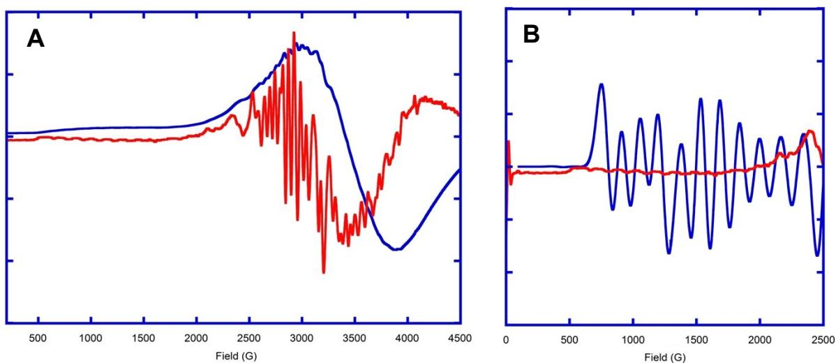
**Figure S5.** **(A)** EPR spectrum of Tc-loaded **Sn-Al-PO<sub>4</sub>** composite at 2.5 K (blue trace) and its first derivative (red trace). **(B)** Overlay of the first derivative of the experimental spectrum of Tc-loaded **Sn-Al-PO<sub>4</sub>** composite (red trace) with the spectrum simulated using the parameters reported for Tc(IV) in the  $\text{SnO}_2$  cassiterite structure.<sup>1</sup>
