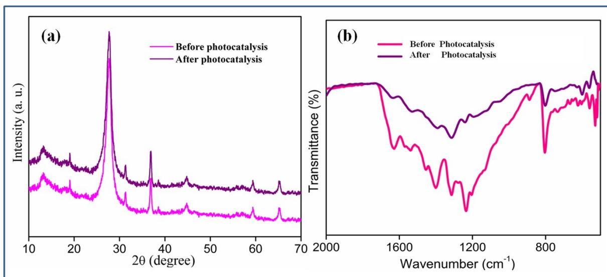
**Fig. S7** (a) XRD and (b) FTIR patterns of g-C<sub>3</sub>N<sub>4</sub>/ Co<sub>3</sub>O<sub>4</sub> (CC) after the cyclic studies.
