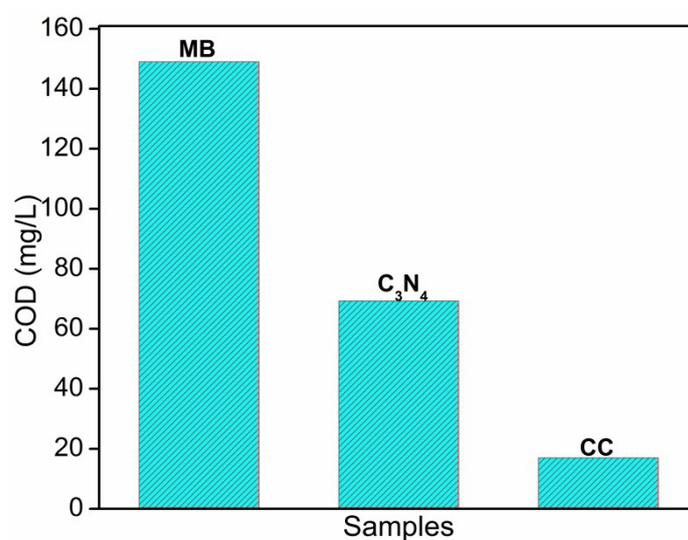
**Fig. S6** COD removal using CC,  $C_3N_4$  and initial MB concentration.
