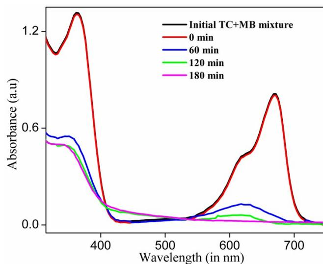
**Fig. S5** UV-Visible degradation patterns of TC and MB in the mixture using CC composite.
