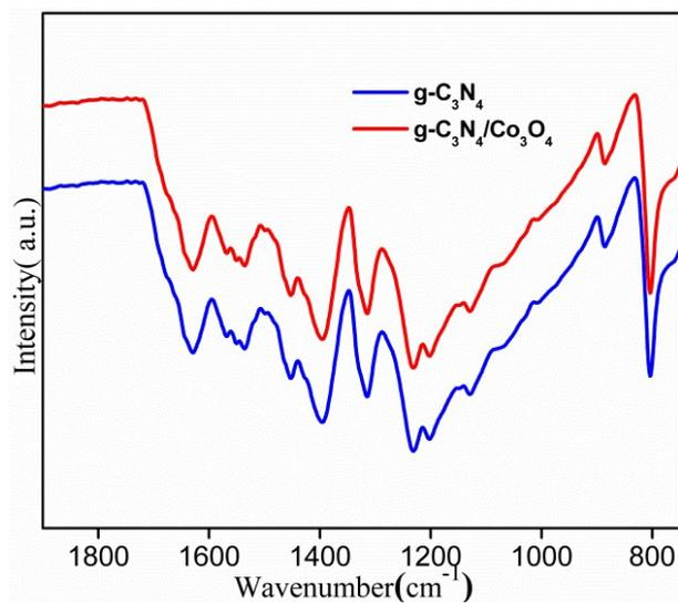
Fig. S3. FTIR spectra of g-C<sub>3</sub>N<sub>4</sub>/ Co<sub>3</sub>O<sub>4</sub> (CC), Co<sub>3</sub>O<sub>4</sub> and g-C<sub>3</sub>N<sub>4</sub>.
