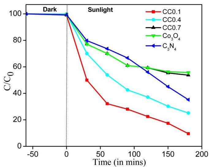
Fig. S4 TC degradation profile of all the composites prepared, pristine C<sub>3</sub>N<sub>4</sub> and Co<sub>3</sub>O<sub>4</sub>.
