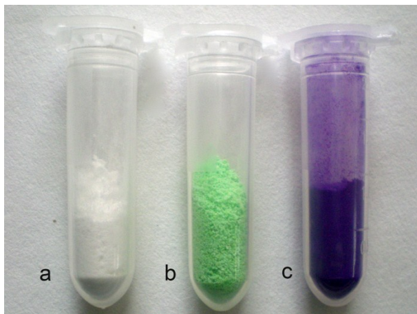
Figure S1 Photo of the MOFs. (a) \text{Zn}_2(\text{bdc})_2\text{dabco} , (b) \text{Ni}_2(\text{bdc})_2\text{dabco} , (c) \text{Co}_2(\text{bdc})_2\text{dabco}
