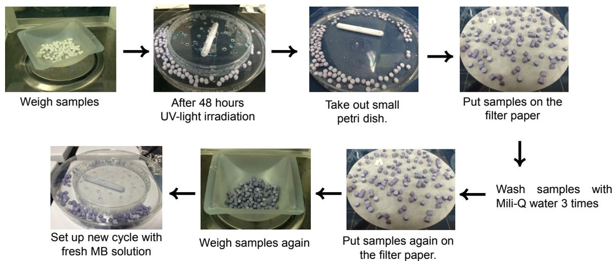
**Fig. S5.** Photographs showing a detailed recycling process for hybrid gel photocatalysts.
