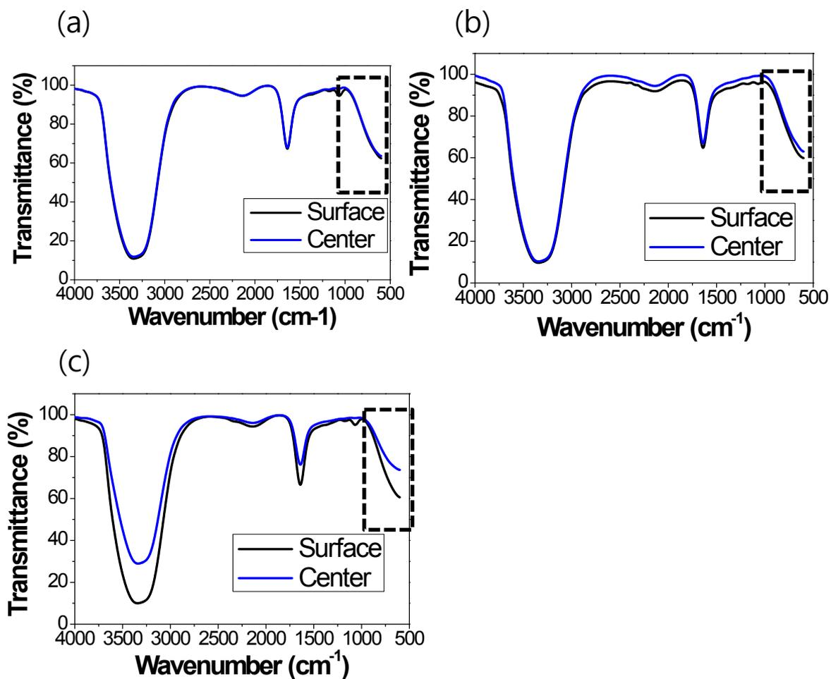
**Fig. S3.** Comparison of FT-IR data taken at surface and center of the dried a hybrid gel for the different initial TiO<sub>2</sub> loading concentration: (a) 1.8, (b) 3.6, and (c) 7.2 wt% .
