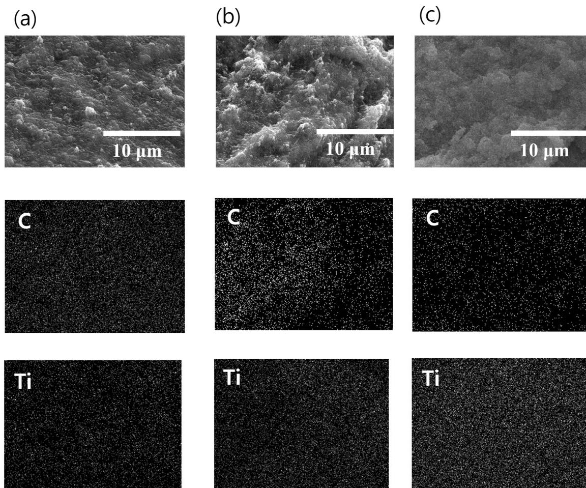
**Fig. S2.** SEM image and corresponding EDX mapping images based on C and Ti atoms for different TiO<sub>2</sub> content: (a) 1.8, (b) 3.6, and (c) 7.2 wt% in a hybrid gel.
