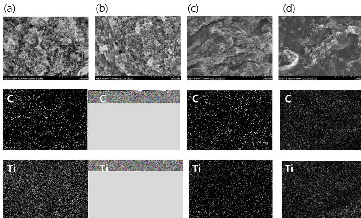
**Fig. S4.** SEM image and corresponding EDX mapping images based on C and Ti atoms for different agarose content: (a) 2.0, (b) 3.0, (c) 4.0, and (d) 5.0 wt% in  $\text{TiO}_2$ /agarose hybrid gel.
