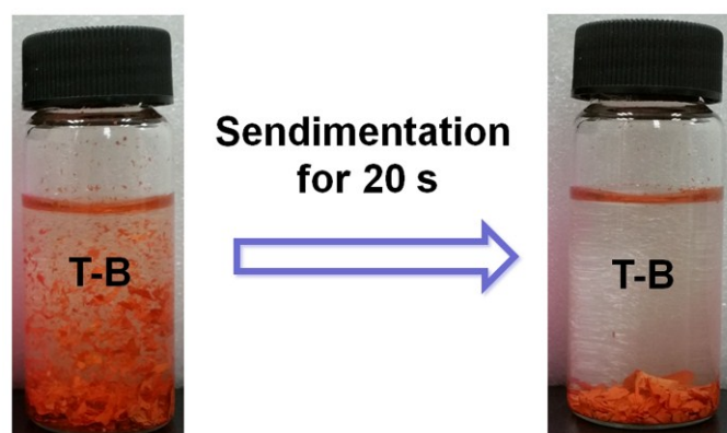
Fig. S10 The easy recycle of \text{Ta}_3\text{N}_5/\text{Bi}_2\text{MoO}_6 by a simple sedimentation.
