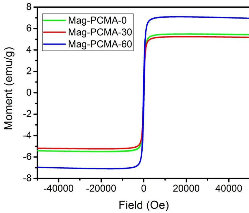
**Figure S2.** The magnetic hysteresis loops of Mag-PCMAs-0, Mag-PCMAs-30, and Mag-PCMAs-60.
