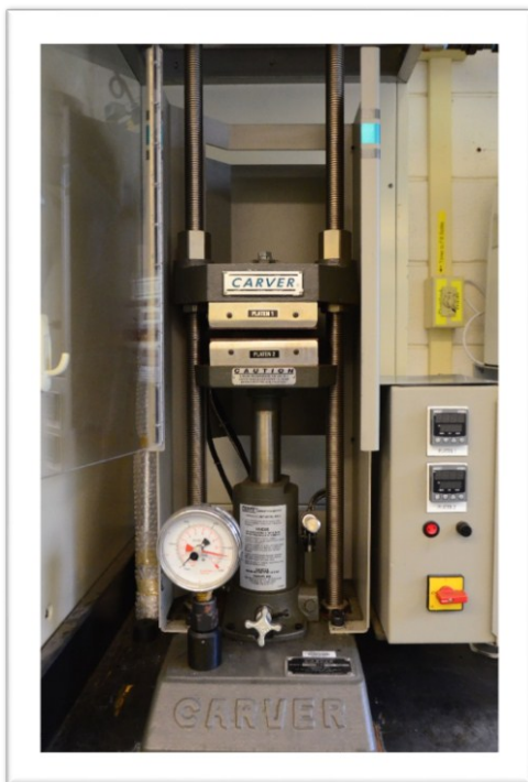
Fig. S1 Pressing machine with temperature control unit.
