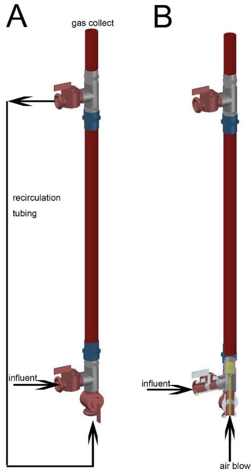
**Fig. S1 – Reactor configuration A. AFMBR, B. AOFMBR and AeMBR. AeMBR and AOFMBR had the same reactor configuration except no GAC was added into AeMBR**
