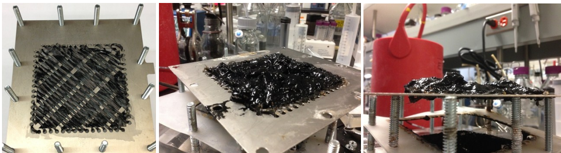
57 Figure S1. Photos of anode fibers: i) initial (left) and ii) after 12-day HRT at high pH (right).
