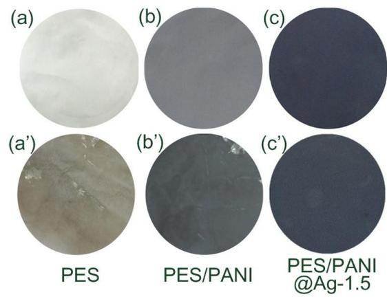
**Fig. S3** The digital photos of membranes before biofouling (a-c), and after biofouling (a'-c').
