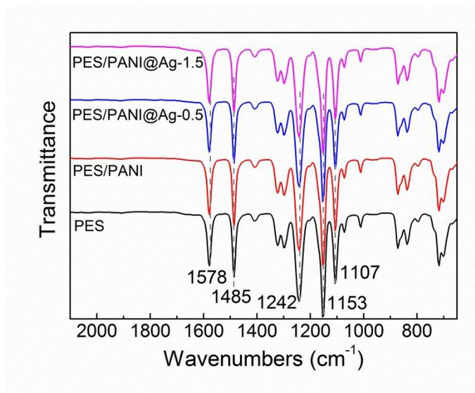
**Fig. S1** ATR-FTIR spectra of PES, PES/PANI and PES/PANI@Ag composite membranes.
