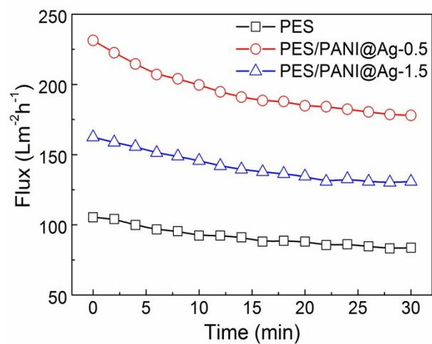
**Fig. S2** The time-dependent pure water fluxes of the membranes during membrane compaction at 0.30 MPa TMP.
