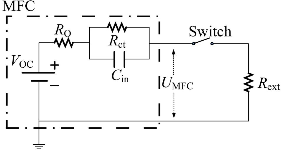
**Fig. S3.** The MFC sensor equivalent circuit model. It consisted of two internal resistors (Ohmic resistance,  $R_o$  and activate resistance,  $R_{ct}$ ) and one internal capacitor ( $C_{in}$ ). Within each cycle, the  $U_{MFC}$  can be divide into  $U_{on}$  when the MFC sensor was connected to the external resistance, and the  $U_{off}$  when the MFC sensor was disconnected to the external resistance.
