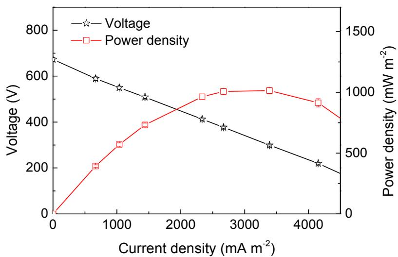
**Fig. S1.** The polarization curves and power density curves of four MFC sensors. Two of them were with the transient-state mode in the following tests, while the remaining two were used as the control.
