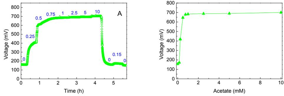
**Fig. S2.** The performance of the MFC sensor operated with an open circuit as a control when fed acetate from 0 to 10 mM. (B) The relationship between the voltage output and the acetate concentration.
