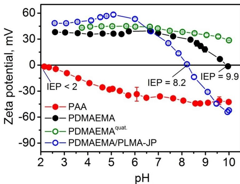
**Figure S3.** Electrophoretic measurements of silica particles covered with polymer shells: silica particles homogeneously decorated with PAA (red circles); silica particles homogeneously decorated with PDMAEMA (black circles); silica particles homogeneously decorated with quaternized PDMAEMA (green circles); PDMAEMA/PLMA Janus particles (blue circles).
