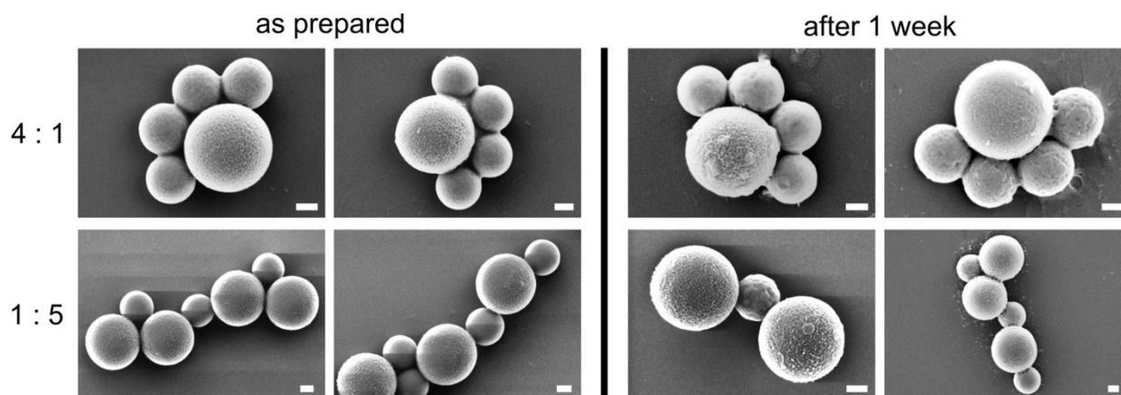
**Figure S6.** Representative SEM images of the micro-clusters assembled from PAA-450 and PDMAEMA/PLMA-JP-1 $\mu$ m directly after dispersion preparation (left), and after imaging the same dispersion in 1 week and additional sonication (right). Upper row: half-raspberry-like micro-clusters (PAA:JP = 4:1); lower row: dumbbell-like micro-clusters (PAA:JP = 1:5). Scale bars: 200 nm.
