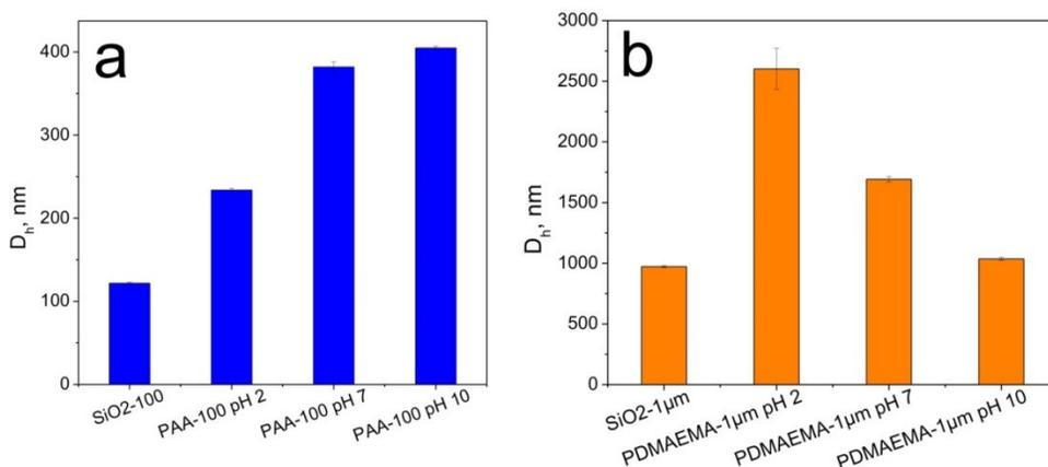
**Figure S4.** Hydrodynamic diameter ( $D_h$ ) of the corresponding undecorated SiO<sub>2</sub> core particles, and (a) PAA-100, as well as (b) PDMAEMA-1µm homogeneously decorated core-shell particles depending on the pH value of the dispersion measured by DLS.
