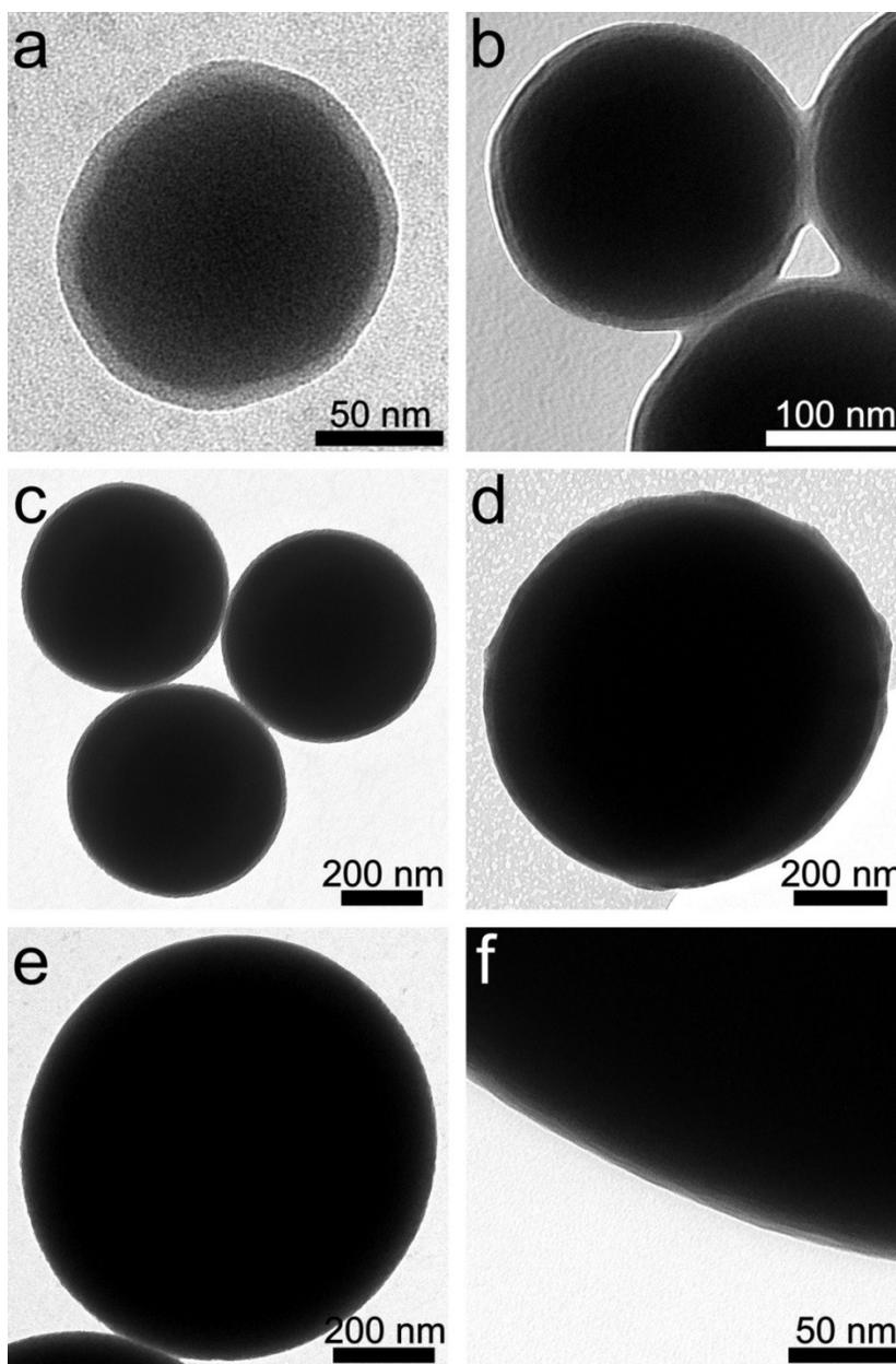
**Figure S1.** TEM images revealing the core-shell structure of the prepared homogeneously decorated as well as Janus hybrid particles: (a) PAA-100; (b) PAA-200; (c) PAA-450; (d) PDMAEMA-1 $\mu$ m; (e, f) PDMAEMA/PLMA-JP-1 $\mu$ m.
