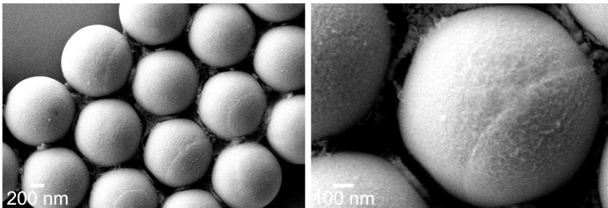
**Figure S2.** SEM images of the PDMAEMA/PLMA-JP-1 $\mu$ m Janus particles.
