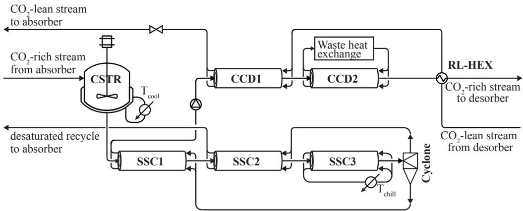
**Fig. 2** conceptual flowscheme illustrating all the heat integration equipment considered in the pinch analysis in Figure 1. The scraped-surface crystallizers (SSC) and the counter-current dissolvers (CCD) enable counter-current heat transfer between suspensions. They can in principle also be realized as a cascade of continuously stirred tank reactors (CSTR).
