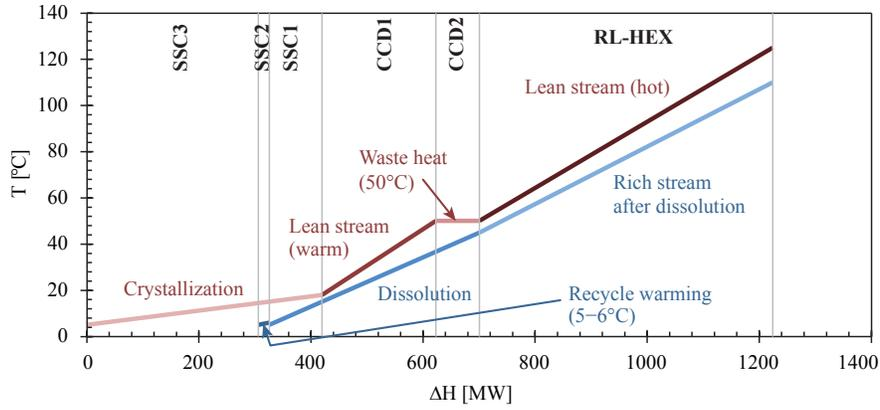
**Fig. 1** Composite curve for the CSF-CAP assuming the optimized operating conditions. See Figure 2 for a detailed flowscheme that enables such heat integration.
