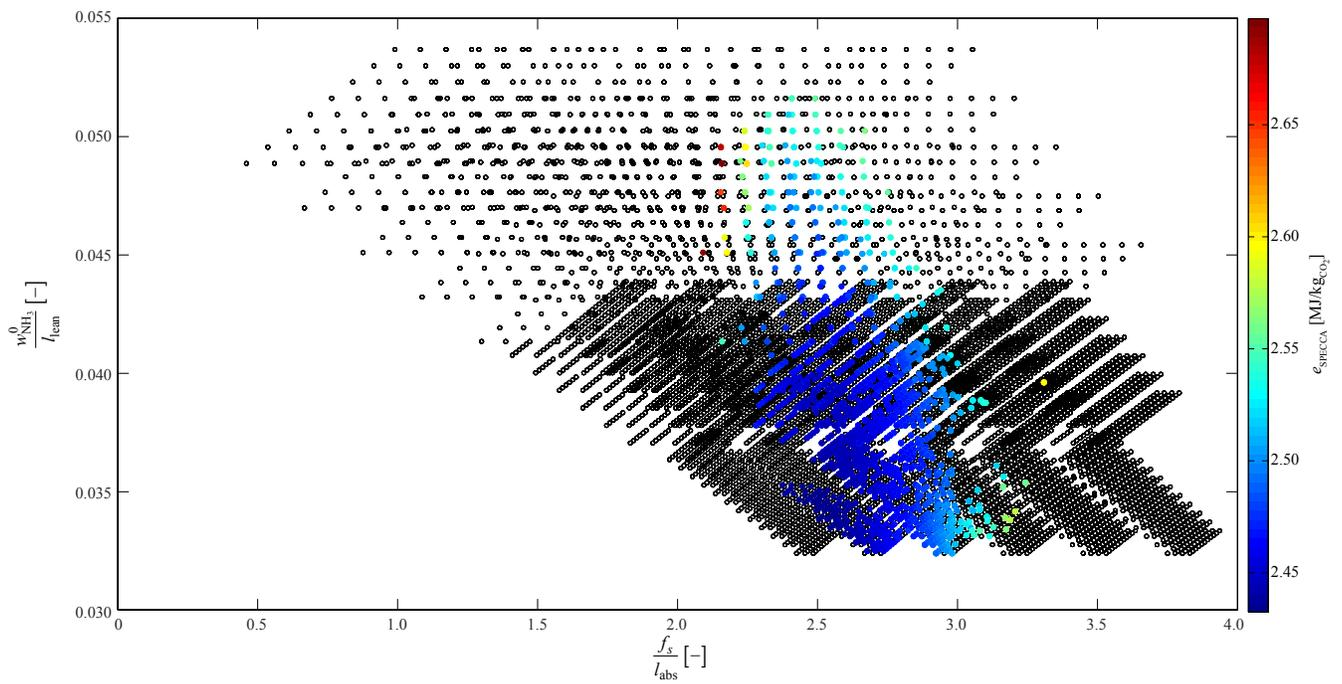
**Fig. 4** Variable range covered by the CSF-CAP simulations. Each point corresponds to one simulation. Black circles represent simulations that did not reach convergence or did not meet the specifications. The coordinates are a combination of the varied input parameters.
