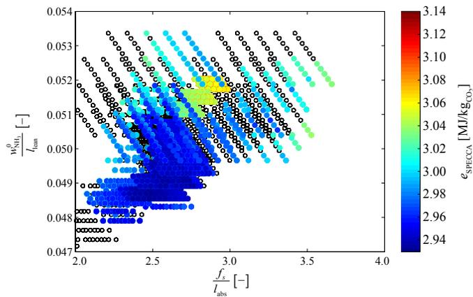
**Fig. 3** Variable range covered by the L-CAP simulations. Each point corresponds to one simulation. Black circles represent simulations that did not reach convergence or did not meet the specifications. The coordinates are a combination of the varied input parameters.
